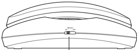
Set **RINGER ON/OFF** to ON to turn the ringer on or OFF to turn the ringer off.
