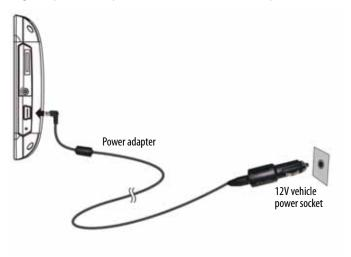
2 Plug the other end of the power adapter into the vehicle's 12V power socket.
