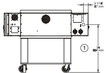
Figure 2-6. MODEL PS536ES DOUBLE OVEN DIMENSIONS
