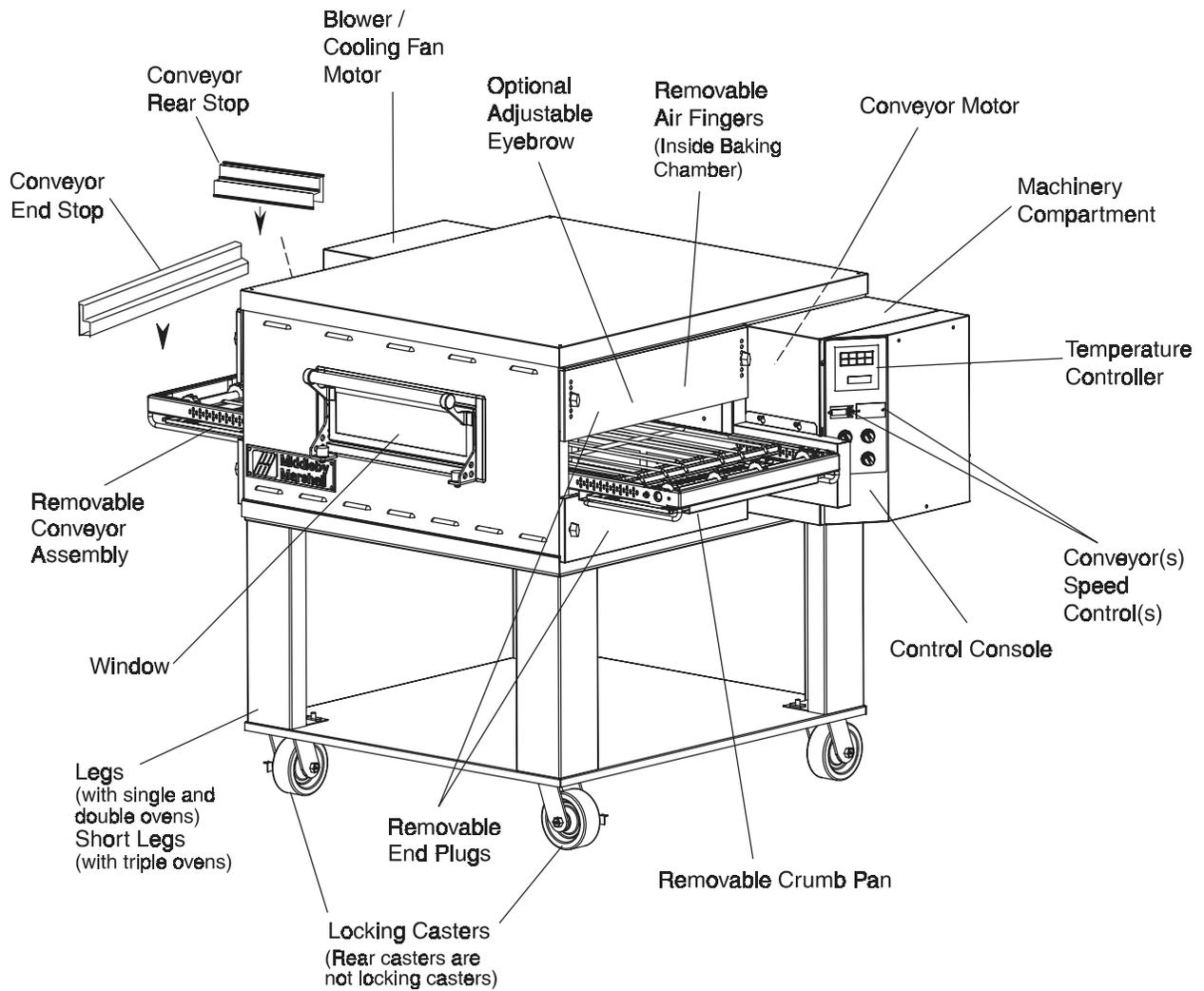
Figure 1-6. PS536ES-Series Oven Components Locations
