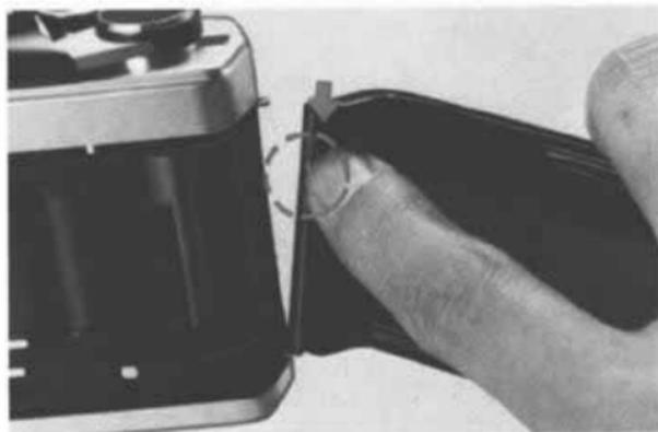
The camera back of the OM-2 is fully interchangeable with the Recordata Back 2, 3 and 250 Film Back 1. To remove the camera back, push down on the release pin as shown. Do not remove the back unless necessary.
