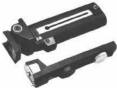
The bounce head can be angled 90° up, 20° down, 60° right and 240° left allowing free choice of bounce and close-up flash photography. Electrical connection with the camera is made via the TTL Auto Cord T and TTL Auto Connector.
