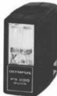
PS200 operates on two 1.5V AA batteries (recycling time approx. 7 sec.) and the PS200 Quick on four AA batteries (2~3 sec.). PS200: 31 x 55 x 64mm (1.2" x 2.2" x 2.5"), 75g. (2.6 oz.) less batteries. PS200 Quick: 32 x 73 x 71mm (1.3" x 2.9" x 2.8"), 95g. (3.4 oz.) less batteries.
