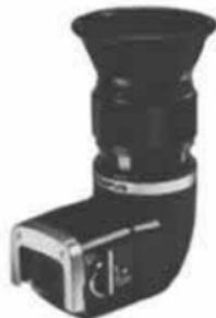
use in low level and 90° angled shots. The two-stage, one-touch switching system offers both a 1.2x magnification image covering the whole screen, and a 2.5x enlargement of the central portion for critical focusing. For photomicrographic use, insert the Eyecoupler between the camera and Varimagni Finder.
