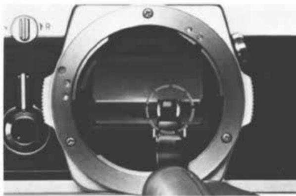
The OM System interchangeable focusing screens provide you with the ultimate in focusing versatility. Optional screens are available to suit virtually every picture-taking situation. The focusing screens come with a special tool. To remove the focusing screen:
