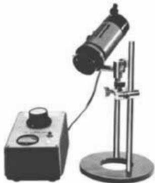
nator Base X-DE, the Illuminator supplies transmitted light. Focusing is adjustable by shifting the bulb filament. A 6V to 8V variable transformer is provided. Eight filters are available in various sizes, including color, black and white, neutral density, etc. for transparent or translucent subjects.
