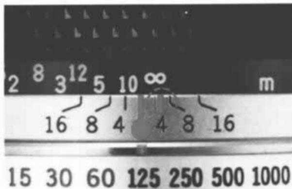
The OLYMPUS OM System Lenses are provided with an infrared index mark engraved in red on the depth of field scale.
