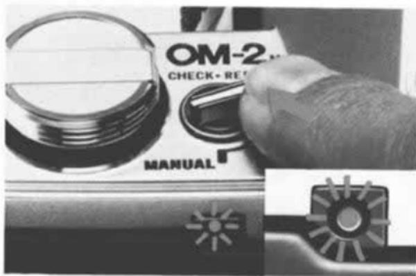
By pressing the selector lever to the "CHECK•RESET" position, you can check the batteries and/or unlock the mirror.
