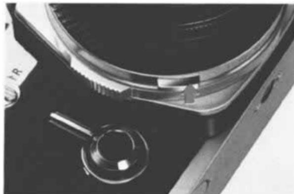
When you wish to see which objects fall within the acceptable zone of sharpness (depth of field), press the preview button on your lens. The diaphragm of the lens will stop down to the preset F stop enabling you to see the depth of field in the viewfinder.
