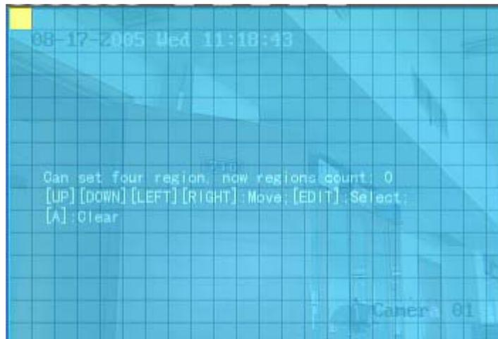
Fig 5.13 Mask area setup
