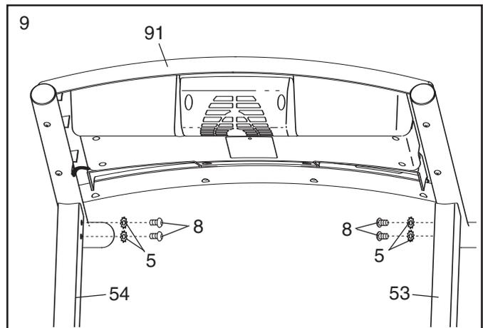
10. Tighten two M8 x 15mm Bolts (8) with two M8 Star Washers (5) into the Uprights (53, 54).
