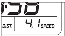
**The upper display**—The upper display can show the elapsed time, the distance that you have walked or run, the approximate number of calories you have burned, or the speed of the walking belt. Press the Display button repeatedly until the upper display shows the information that you are most interested in viewing. Note: While information is shown in the upper display, the same information will not be shown in the lower left or lower right display.
