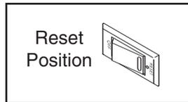
**IMPORTANT:** The console features a display demo mode, designed to be used if the treadmill is displayed in a store. If the displays light as soon as you plug in the power cord and switch the circuit breaker to the reset position, the demo mode is turned on. To turn off the demo mode, hold down the Stop button for a few seconds. If the displays remain lit, see **THE INFORMATION MODE** on page 17 to turn off the demo mode.
