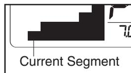
The height of the flashing segment indicates the speed setting for the current segment. At the end of each segment, a series of tones will sound and the next segment of the profile will begin to flash. If a different speed or incline setting is programmed for
