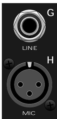
**G. LINE** - Plug your instrument in here. This 1/4 inch TRS balanced input jack suited for use with items having a line level output such as high impedance microphones, keyboards, drum machines, outboard effects, etc. It accepts both balanced and unbalanced cables
