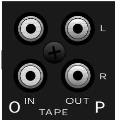
**O. TAPE IN** - Unbalanced phono (RCA) input jacks designed for use with a tape player, CD player, etc. These jacks sum the stereo left and right input signal to a mono signal useful for playing prerecorded music. The *tape/effects return to main* and *tape/effects return to monitor* control the volume to these buses respectively.
