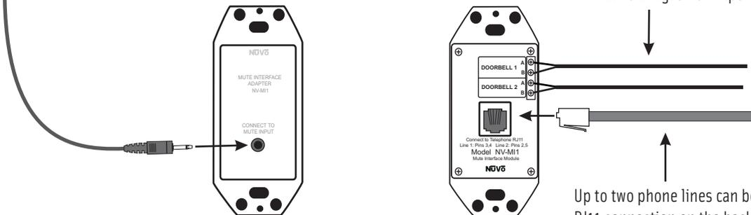
Up to two phone lines can be brought into the RJ11 connection on the back of the MI1. The voltage from the phone ringer will trigger the NuVo System to mute.
