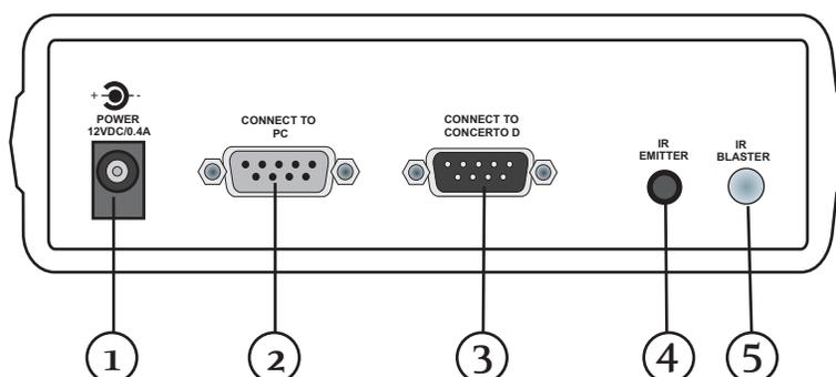
1. **AC Power:** A standard 12-volt power supply is included in the Learning Station Package. This will supply the necessary AC power for IR learning and testing.
