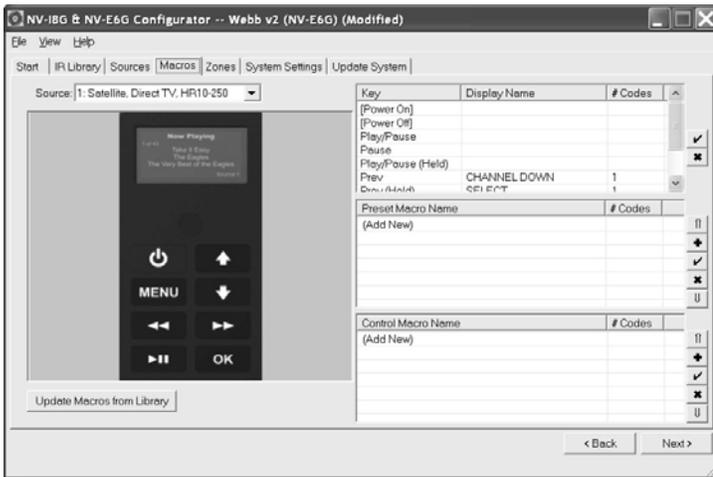
If the component had default keys defined in the IR Library, single IR code macros will be automatically created for each key. Hovering the mouse over each key in the Control Pad picture on the left side of the screen will bring up a tool-tip displaying the name of the macro assigned to that key. Clicking on the key highlights the macro on the right side of the screen.
