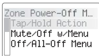
**Advanced:** Within the System settings menu are advanced functions intended for installers. The item is preceded by an asterisk and grayed which requires that the OK button is held for six seconds before the advanced functions are accessible, Fig. 50.
