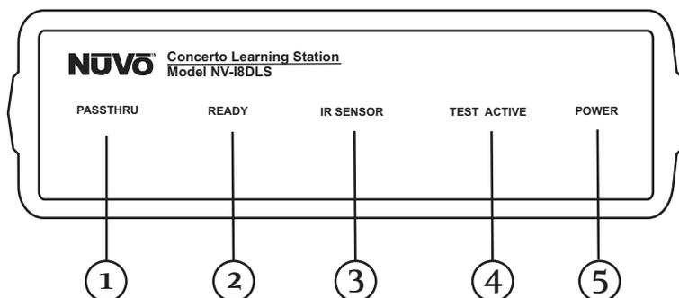
1. **PASSTHRU:** This LED (light emitting diode) remains lit when the Interface box is actively passing IR information through the system.
