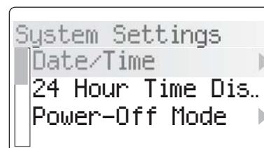
**Date/Time:** The Essentia has an internal clock that allows each Control Pad to display the current time. Within this menu you can easily set **Year, Month, Day, Hour, and Minute.**
