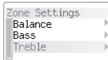
**Balance:** This controls the level of audio going to the left and right speakers. In some cases, when the listening area is not absolutely centered between the speakers, it is useful to adjust the center listening point left or right. This menu option gives the ability to adjust the sound left or right up to 18 steps in either direction.
