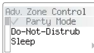
**Party Mode:** This setting is turned on and off with the OK button. When selected all the configured zones in the system will turn on and that Control Pad becomes the Host for the entire house. This function is defeated in an individual zone by initiating a function on that zone's Control Pad.
