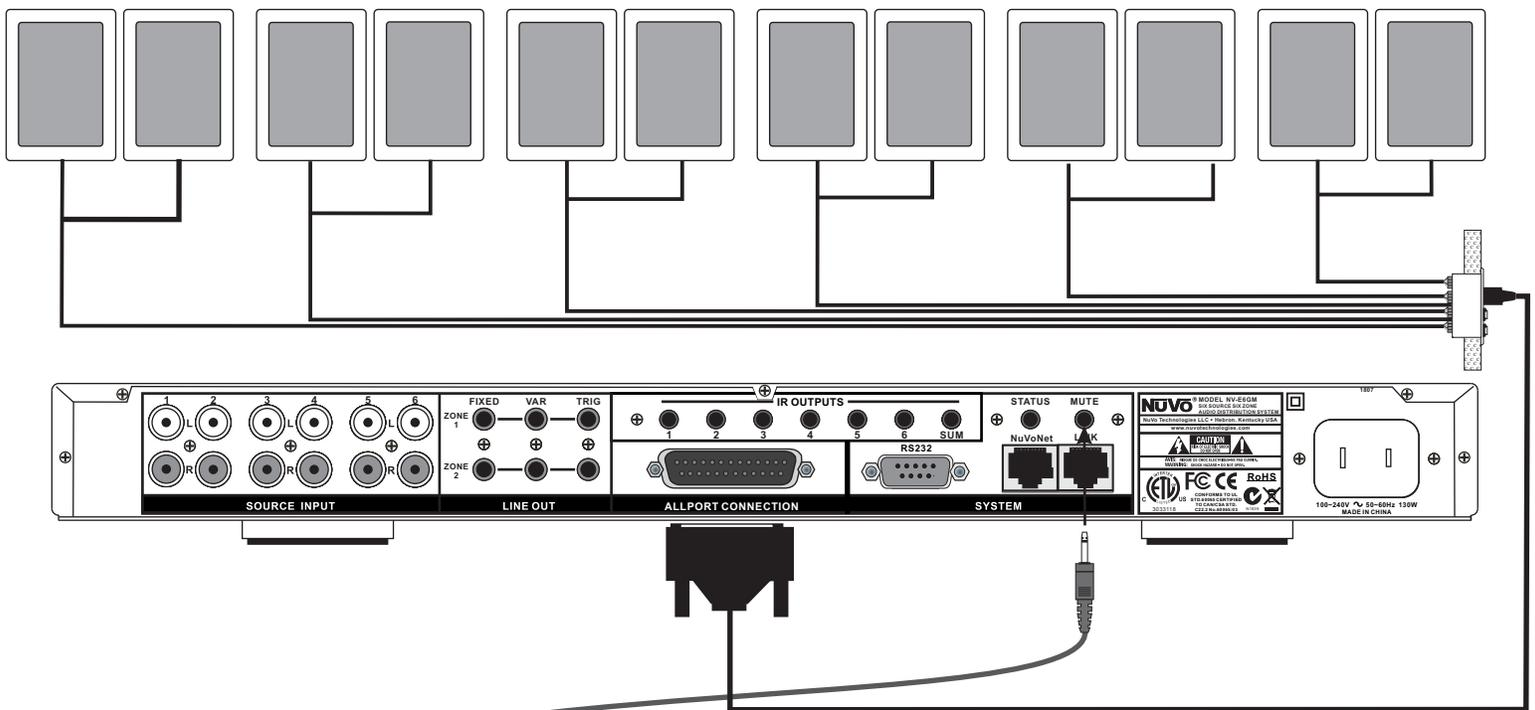
The MI1 connects to the NuVo amplifier using a standard mono patch cable with a mini-plug on each end. Plug one end into the MUTE input on the back of the amplifier and the other end into the input on the front of the MI1.
