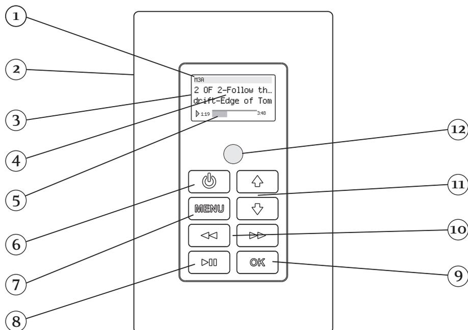
1. **Source Indicator:** This indicates the current audio source playing in that zone. Source names can be customized in the Configurator Software with a three-character designation.
