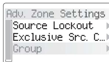
**Source Lockout:** Any source selected in this menu will be locked from access within that zone.
