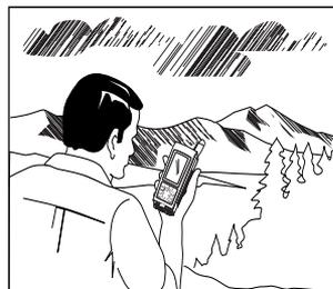
**Holding the Receiver.** Your MAP 410 is designed to fit comfortably in your hand. Hold the receiver in the palm of your hand with the antenna pointing towards the sky.
