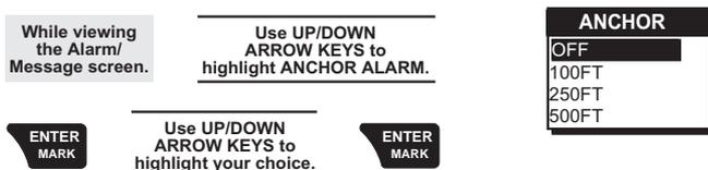
The beeper will sound when the GPS position is at a distance greater than the distance you have chosen. The alarm will sound until you turn it off or the condition is corrected. The default setting is OFF.
