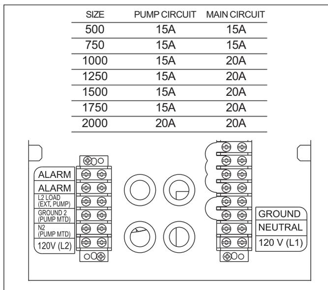
Figure 15. Field Wiring.
