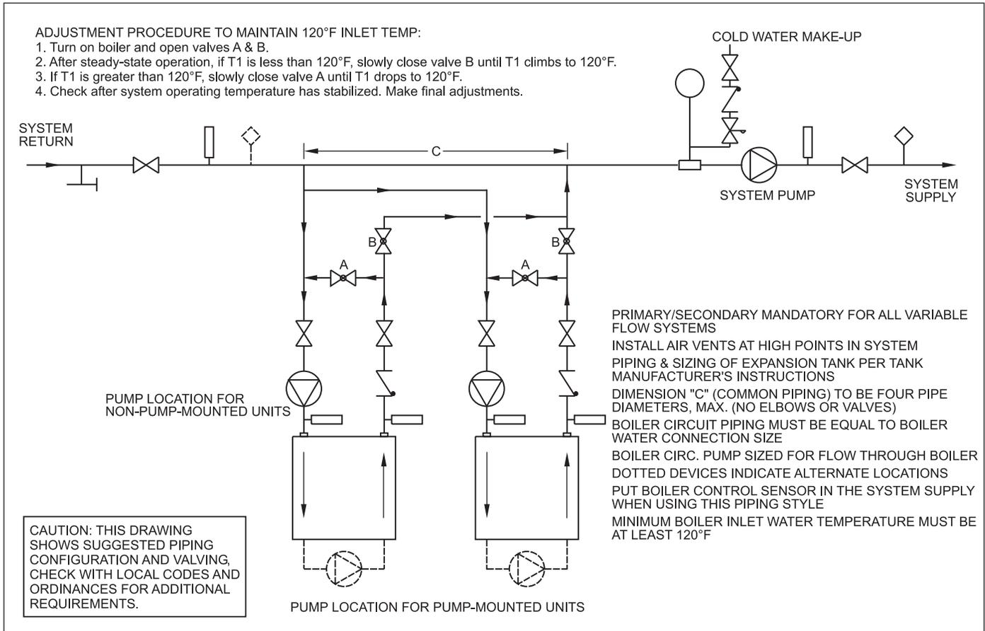
Figure 10. Hydronic Piping - Primary-Secondary, Reverse-Return, Low Temperature.
