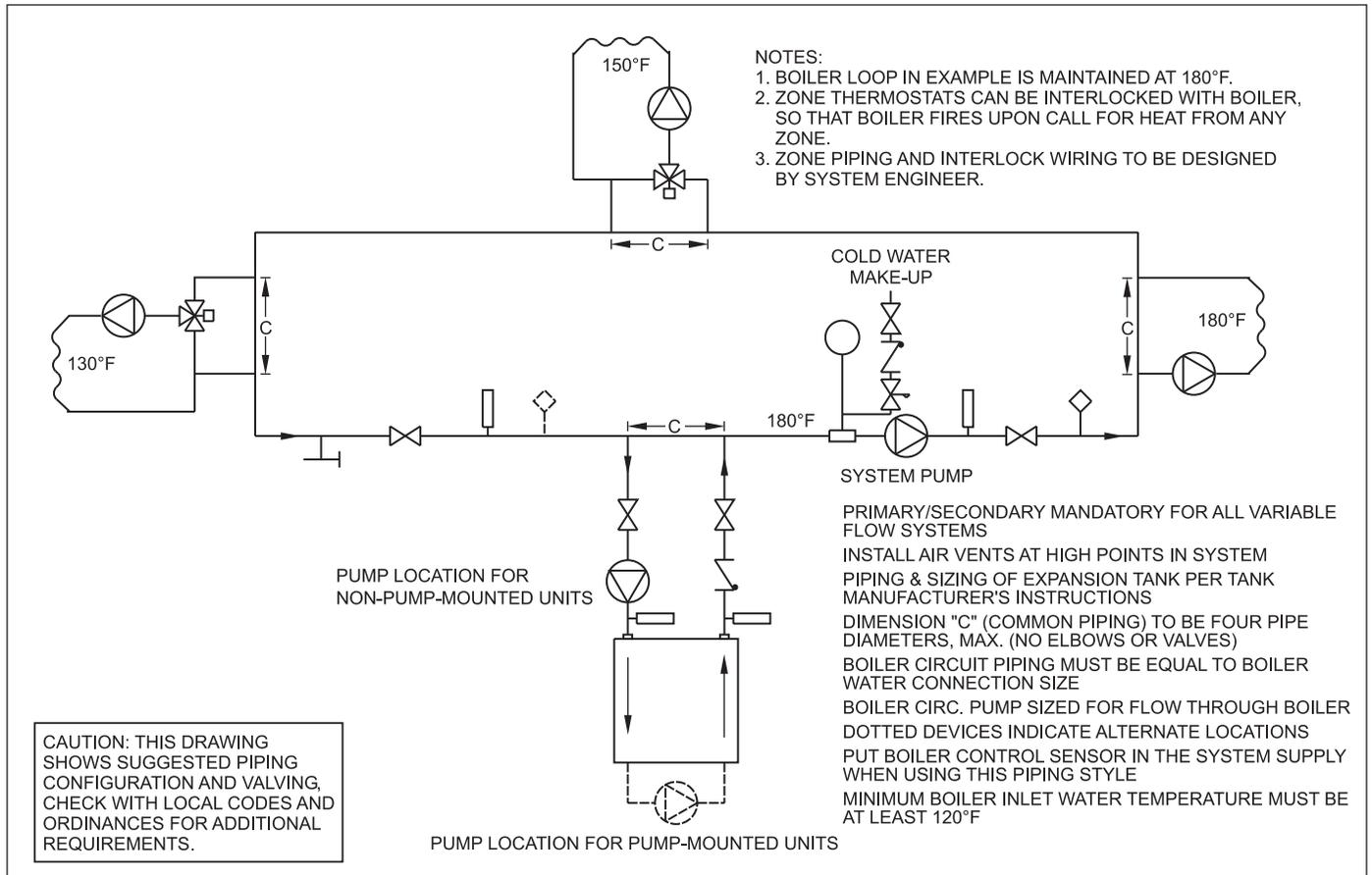
Figure 8. Hydraulic Piping — One Boiler, Multi-Temperature System.
