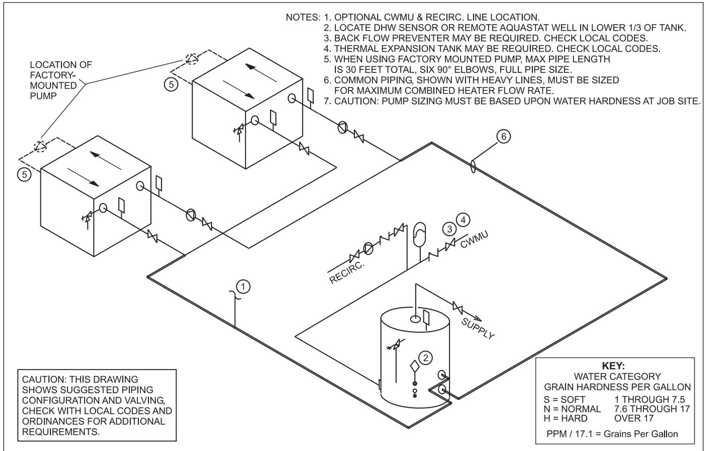
Figure 12. Water Heater Piping — Multiple Heaters, One Tank.
