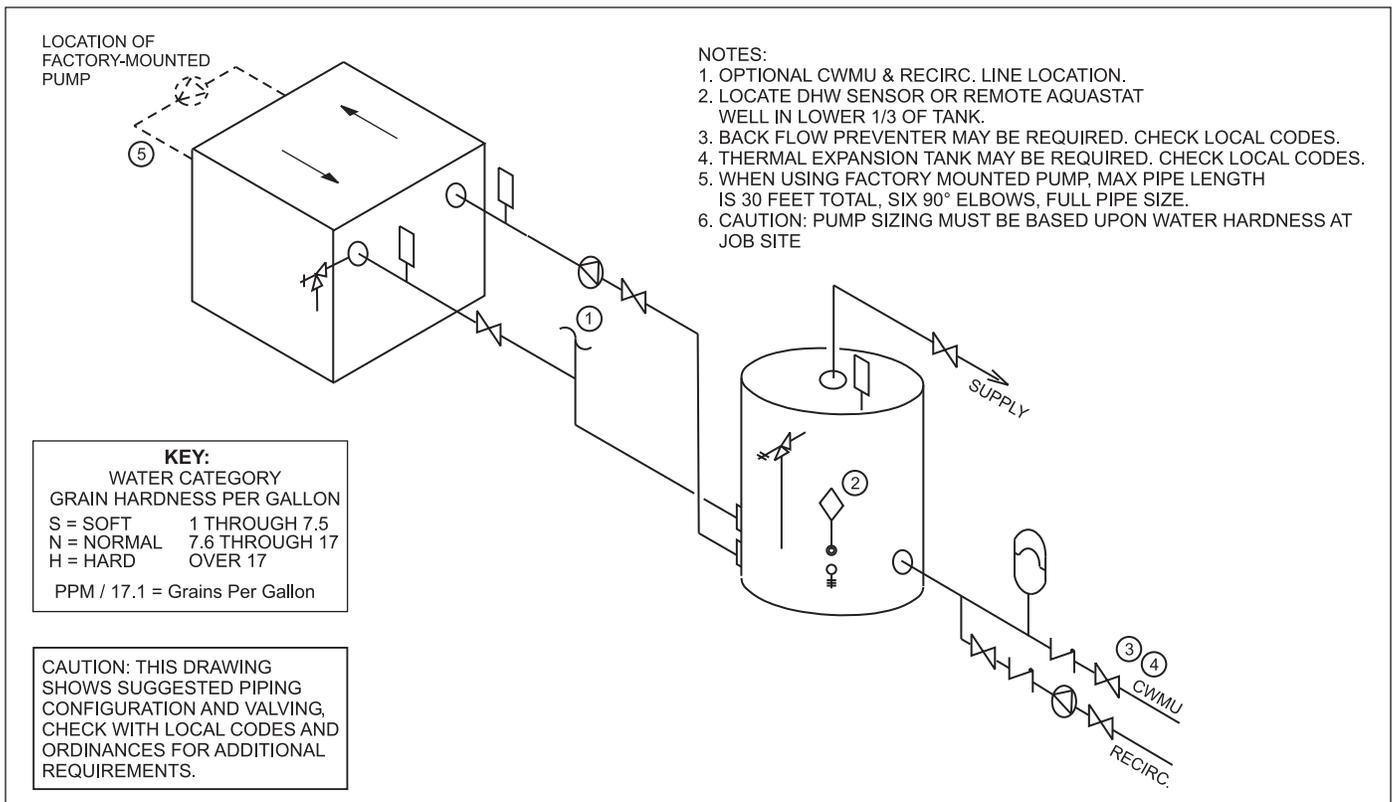
Figure 11. Water Heater Piping — One Heater, One Tank.
