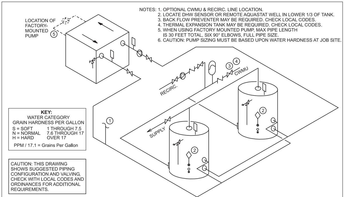
Figure 13. Water Heater Piping — One Heater, Multiple Tanks.
