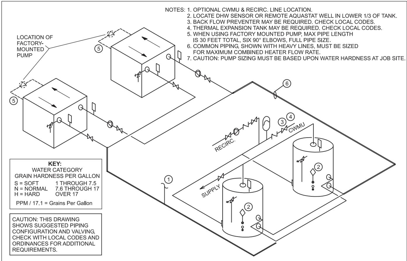
Figure 14. Water Heater Piping — Multiple Heaters, Multiple Tanks.
