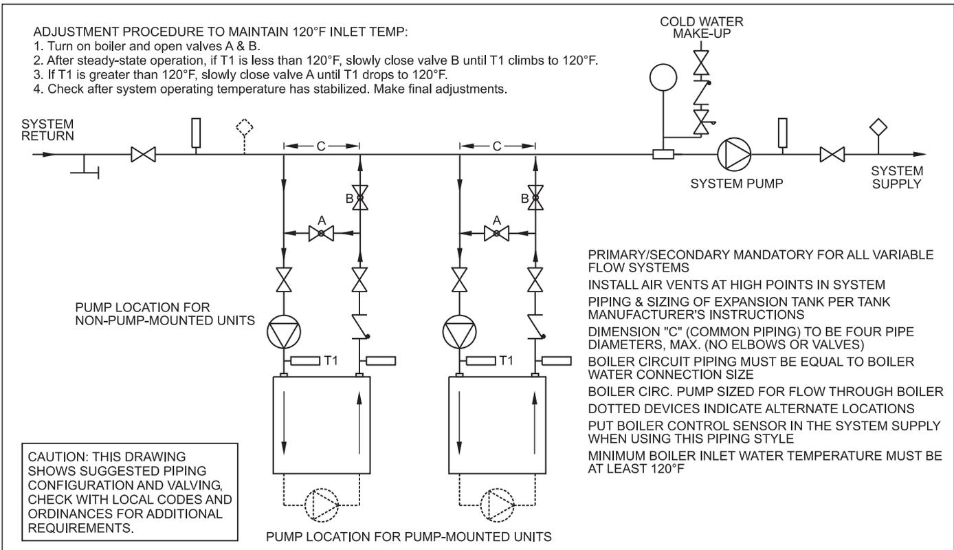
Figure 7. Hydraulic Piping — Multiple Boilers, Low Temperature System.
