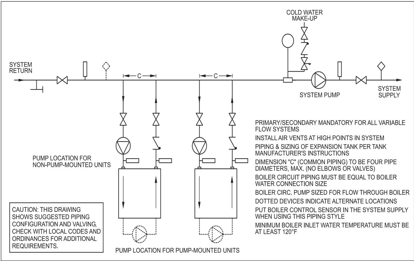
Figure 6. Hydraulic Piping — Multiple Boilers, Primary Secondary System.
