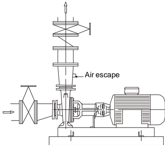
**Priming of a flooded pump**
