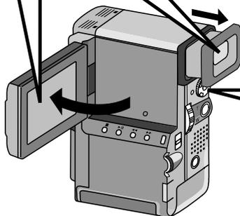
To turn on the camcorder, first turn the Power Dial to any operation mode except "OFF", then pull out the viewfinder fully or open the LCD monitor. When turning the Power Dial from "OFF" to "A" or when turning it from "OFF" to "PLAY", press and hold the lock button located on the dial.
