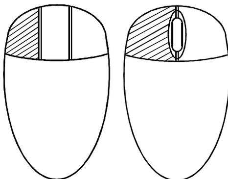
To select a computer in **EXCLUSIVE** mode, use the left hand mouse button together with the SHIFT key on the keyboard. To select a computer in **VIDEO ONLY** mode use the left hand mouse button together with the CTRL key on the keyboard.
