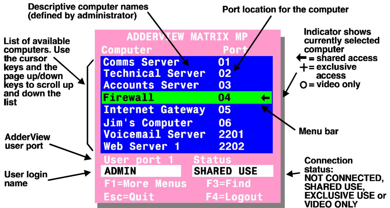
To connect to a computer, place the menu bar over the computer name using a combination of the up and down cursor keys and the page up / page down keys.
