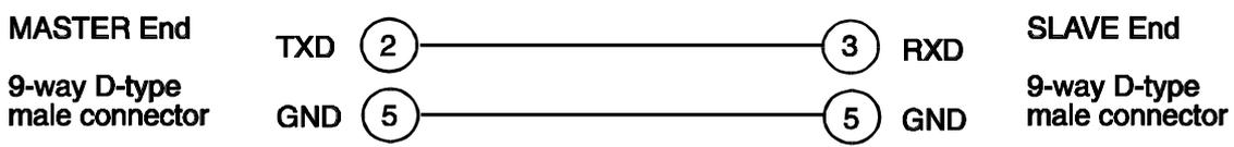
The pinout for a “daisy chain” RS232 cable for more than 2 units is shown below:
