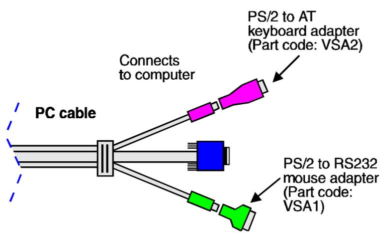
**Cables for connection to Sun computers with 8-pin keyboard/mouse connectors:**
