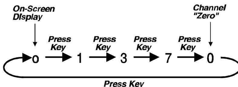
Action of the COMPUTER key if the front panel controls have been disabled.
