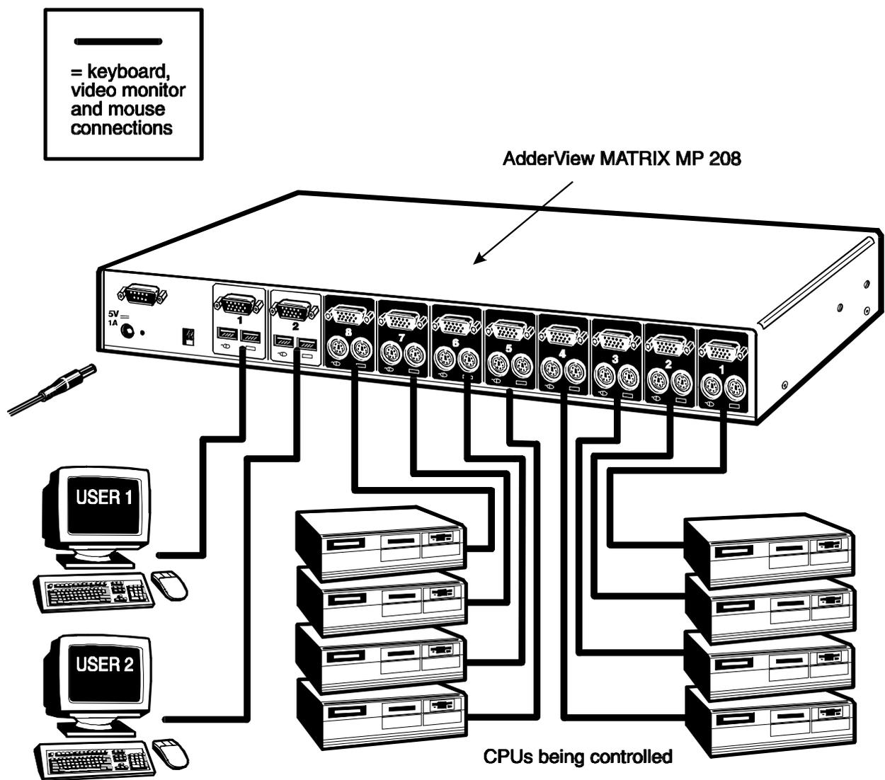
Fig. 4 - A typical installation using a single AdderView MATRIX MP 208
