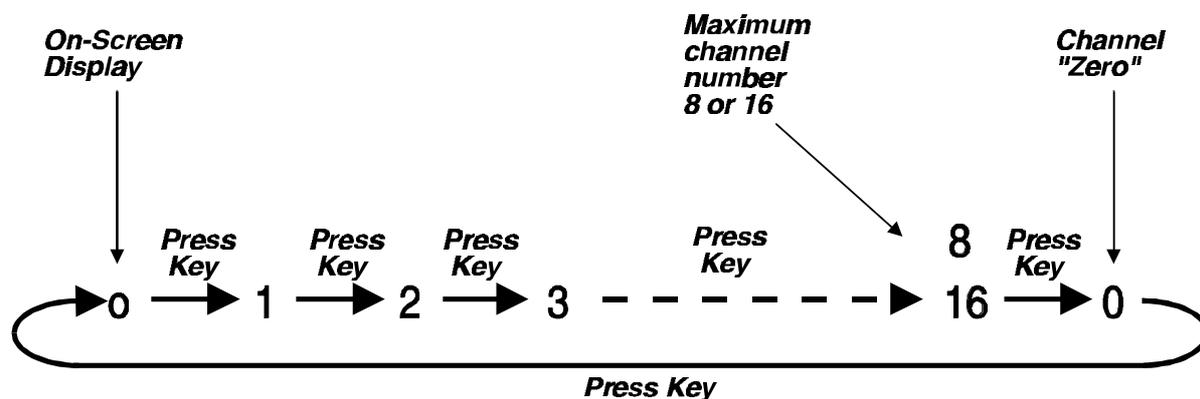
Action of the COMPUTER key if the front panel controls are enabled, security has been set and the current logged in user only has access to computer ports 1,3 and 7
