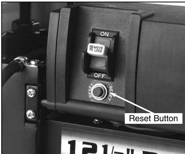
Figure 5. Location of switch and reset button.
