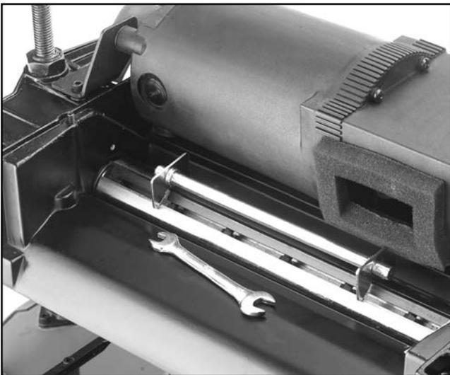
**Figure 10.** Knife gauge positioned on cutterhead.
