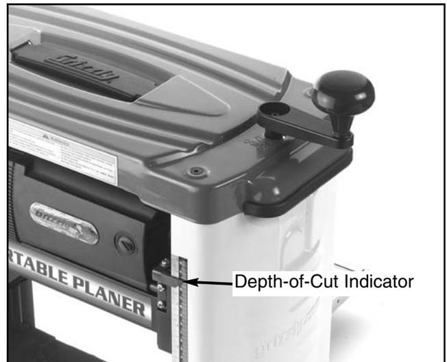
Figure 6. Depth-of-cut handle and indicator.
