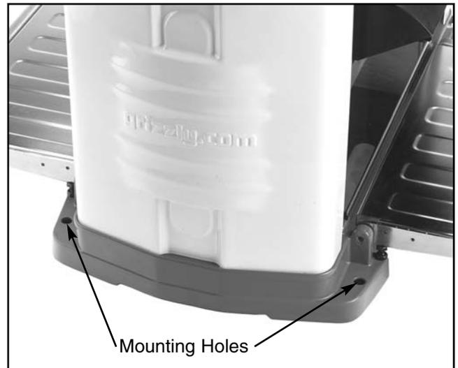
**Figure 4.** Mounting hole location.
