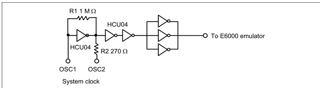
**Figure 9 Oscillator Circuit**
