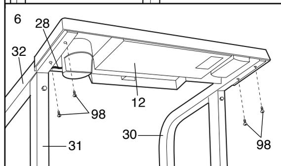
**Tighten all parts used in steps 3 and 5. Then, tighten the 1 1/4" Screws (98) used in this step.**
