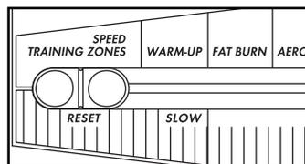
Next, slowly move the speed control until the walking belt begins to move at slow speed. Carefully step onto the walking belt and begin exercising. Change the speed of the walking belt as desired by moving the speed control.
