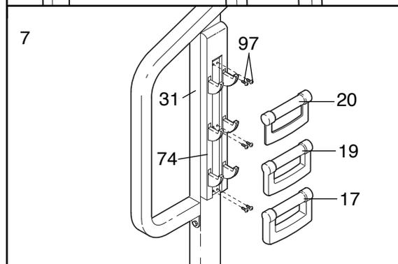
Put the two 2-lb. Weights (20) on the upper hooks on the Weight Racks (74), the 3-lb. Weights (19) on the center hooks, and the 4-lb. Weights (17) on the lower hooks.
