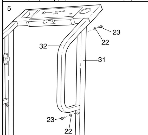
Thread a 1/4" x 1" Bolt (23) with a 1/4" Washer (22) only a couple of turns into the lower end of the Right Handrail (32) and the right Upright (31). **Do not tighten the Bolt yet.**
