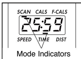
If desired, the Speed, Time, Distance, Fat Calories or Calories mode can be individually selected. Press the MODE button repeatedly until the desired mode indicator appears. Make sure that there is not a mode indicator by the word SCAN.
