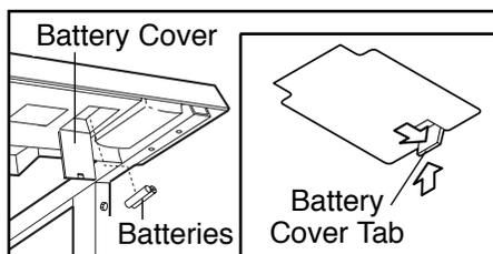
ment, with the negative (–) ends of the batteries touching the springs. Close the battery cover, push up on the tab, and then push the tab forward as shown in the inset drawing. Be sure that the tab locks into place.
