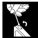
To re-record on a protected tape, cover the holes with adhesive tape.
