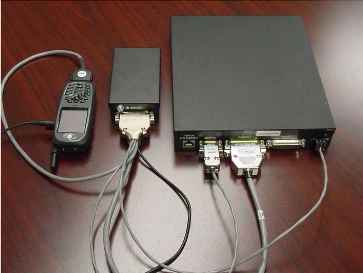
Figure 3 Connections between IP-223 and NI223plus
