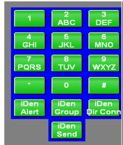
Figure 7 - Manual DTMF key layout with iDen® commands
