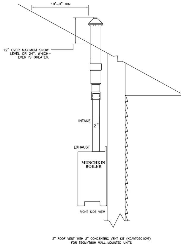
**\*\*IMPORTANT NOTE:** All vent pipes must be glued, properly supported, and the exhaust must be pitched a minimum of a 1/4" per foot back to the heater (to allow drainage of condensate).
