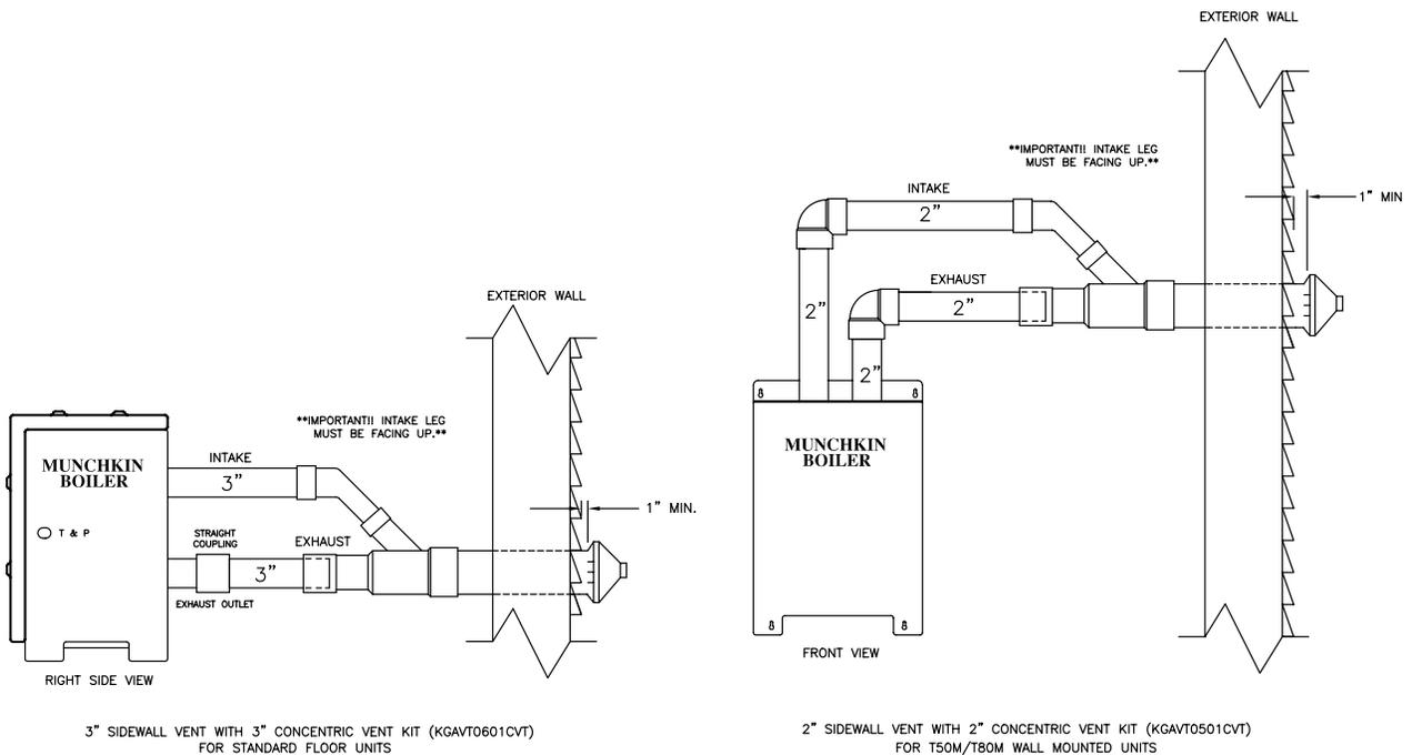
**\*\*IMPORTANT NOTE:** All vent pipes must be glued, properly supported and the exhaust must be pitched a minimum of a 1/4" per foot back to the heater (to allow drainage of condensate).
