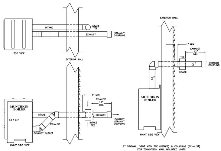
2" SIDEWALL VENT WITH TEE (INTAKE) & COUPLING (EXHAUST) FOR T50M/T80M WALL MOUNTED UNITS
