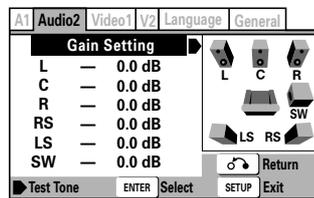
To help you gauge the correct gain levels, set the **Test Tone** to **On** (test tone from just that speaker) or **Auto** (test tone from each speaker in turn, excluding the subwoofer) then adjust the gain so that all speakers appear to be the same volume from your listening position.
