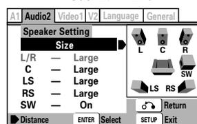
The graphic on the right of the screen represents your speaker setup, with the currently selected speaker's name highlighted in blue, and the speakers set to **On** highlighted in yellow.
