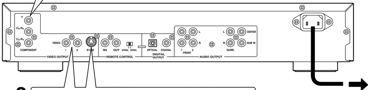
**2** If a component input is not available to you, connect this player to your TV or AV receiver using either the **VIDEO** or **S-VIDEO** jacks.
