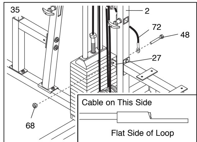
36. **Important:** Follow all three Cables from end to end and make sure they rest in the grooves of all Pulleys and that both the Cables and the Pulleys move smoothly.
