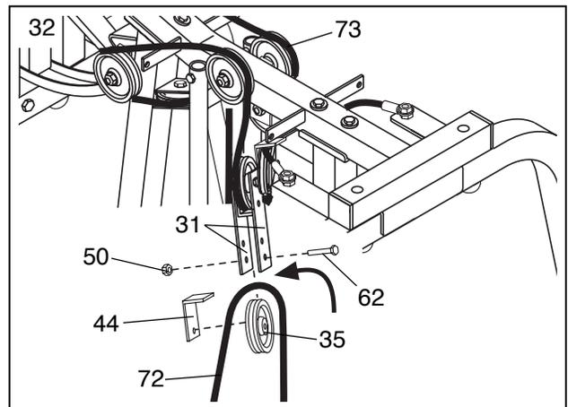
33. Remove the 3/8" Nylon Locknut (50) that was threaded onto the 3/8" x 4 3/4" Bolt (65) in step 31.
