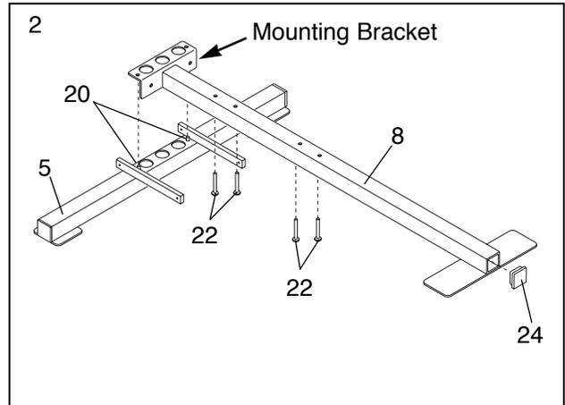
3. Press a 2" Square Inner Cap (24) into the end of the Press Base (4).
