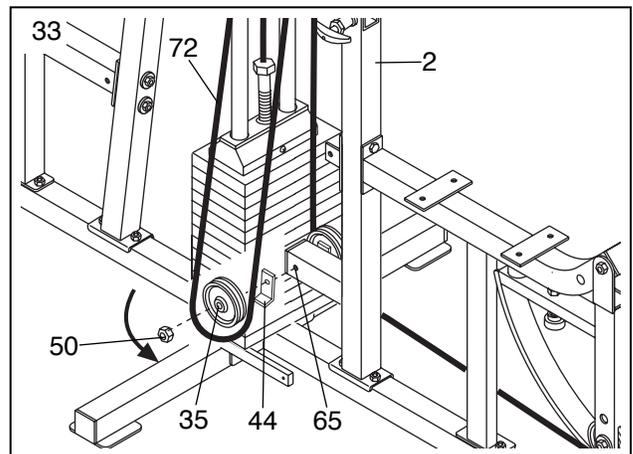
34. Wrap the Low Cable (72) around a 3 1/2" Pulley (35) in the direction shown. Attach the Pulley and a Cable Trap (44) to the "I"-plates (31) hanging from the Short Cable (97). Secure the Pulley and Cable Trap with a 3/8" x 2" Bolt (62) and a 3/8" Nylon Locknut (50).
