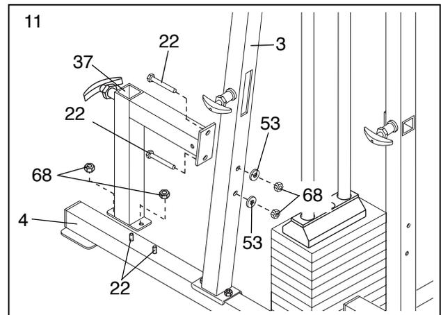
Insert two 5/16" x 2 1/2" Carriage Bolts (22) through the bracket on the Press Seat Upright (37) and through the holes in the Press Upright (3). Slide a 5/16" Flat Washer (53) onto each Bolt. Hand tighten a 5/16" Nylon Locknut (68) onto each Bolt. **Do not tighten the Nylon Locknuts yet.**
