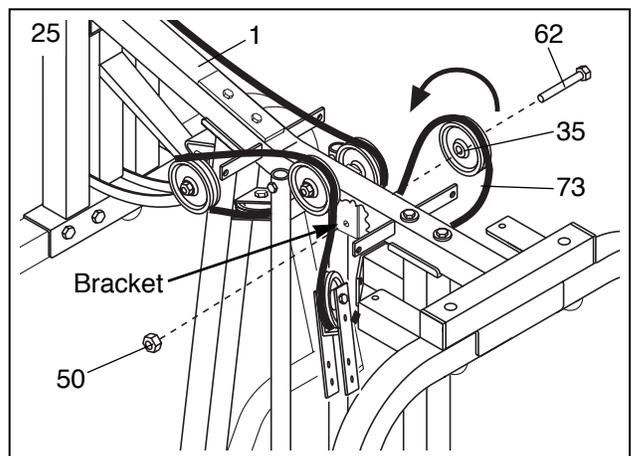
26. Thread the bolt at the end of the High Cable (73) a couple of turns into the top of the Weight Tube (77). This is to prevent the High Cable from falling down during the following steps. It will be permanently attached in step 36.
