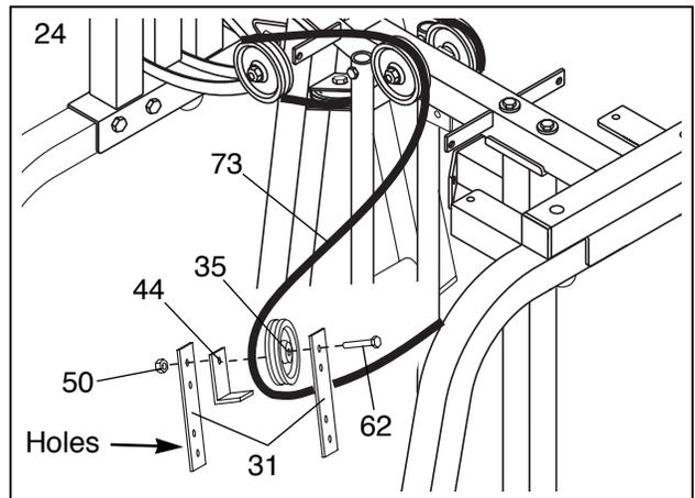
25. Wrap the High Cable (73) around a 3 1/2" Pulley (35) in the direction shown.
