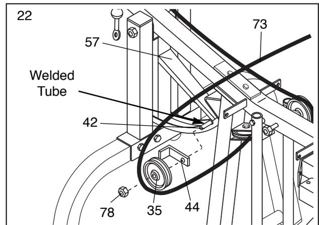
23. Remove the 3/8" Nylon Locknut (50) attached to the 3/8" x 5" Bolt (42) in step 19. Wrap the High Cable (73) around a 3 1/2" Pulley (35) in the direction shown.
