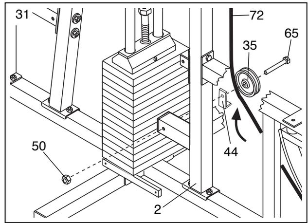
32. Wrap the Low Cable (72) around a 3 1/2" Pulley (35) in the direction shown.
