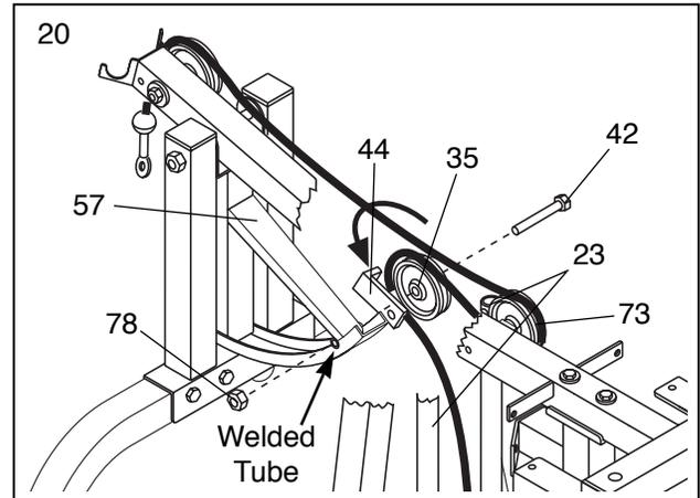
21. Feed the bolt at the end of the High Cable (73) through the indicated bracket on the Press Upright (3) from the direction shown.
