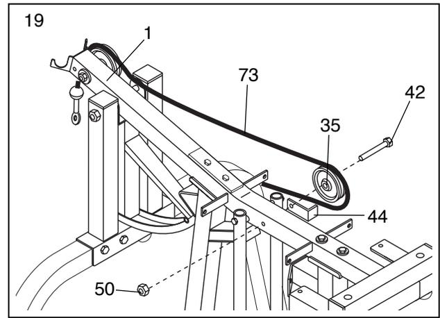
20. Route the High Cable (73) in between the two Weight Guides (23). Wrap the High Cable around a 3 1/2" Pulley (35) in the direction shown.
