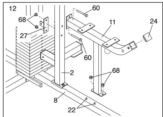
Insert two 5/16" x 2 3/4" Bolts (60) through the bracket on the Butterfly Seat Frame (11) and through the holes in the Butterfly Upright (2). Orient the Support Bracket (27) as shown in the drawing (the horizontal arm of the bracket must be on the side facing away from you in the drawing) and slide it onto the Bolts. Hand tighten a 5/16" Nylon Locknut (68) onto each Bolt. **Tighten all Nylon Locknuts used in steps 6 through 12.**
