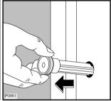
Remove the polystyrene block from the bottom of the machine and release the two plastic bags. Very carefully slide out the left polythene bag, removing it towards the right and then downwards.
