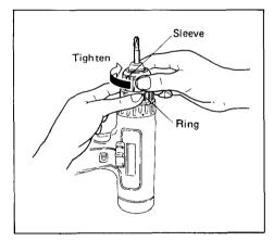
To remove the bit, push the sleeve up toward the "FREE" side and turn the sleeve counterclockwise while holding the ring with your other hand.
