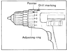
Before actual operation, drive a trial screw into your material or a piece of duplicate material to determine which torque level is required for a particular application.
