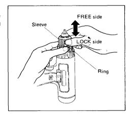
Place the bit in the chuck as far as it will go. Hold the ring firmly and turn the sleeve clockwise to tighten the chuck. Then push the sleeve down toward the "LOCK" side. See illustration.
