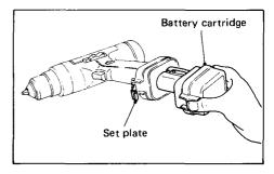
Do not use force when inserting the battery cartridge.
