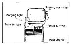
If the charging light does not come on, press the reset button (yellow) first, then the start button (red). If the charging light goes out within 10 seconds even after pressing the reset button and start button a couple of times, the battery cartridge is dead. (CAUTION: Wait for more than 5 seconds after the charging light goes out to press the reset button again.) Replace it with a new one. When the charging light goes out after about one our, you may remove the fully charged battery cartridge.
