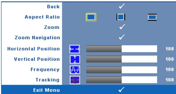
**ASPECT RATIO**—Allows you to select the aspect ratio to adjust how the image appears.
