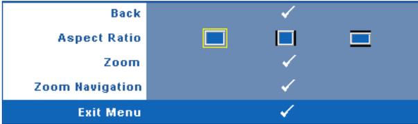
**ASPECT RATIO**—Allows you to select the aspect ratio to adjust how the image appears.
