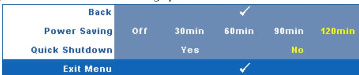
**POWER SAVING**—Select **Off** to disable Power Saving mode. By default, the projector is set to enter power saving mode after 120 minutes of no activity. A warning message appears on screen showing a 60-second countdown before switching to power saving mode. Press any key buttons during countdown period to stop power saving mode.
