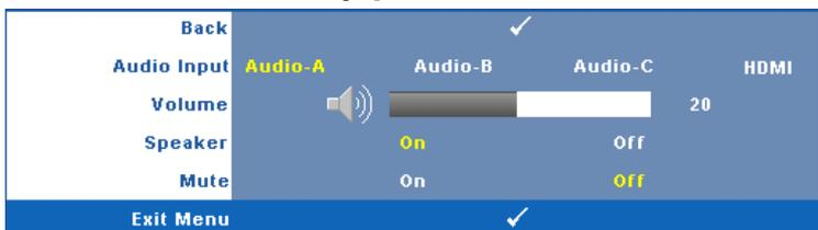
**AUDIO INPUT**—Select the Audio input source, options are: Audio-A, Audio-B, Audio-C, and HDMI.
