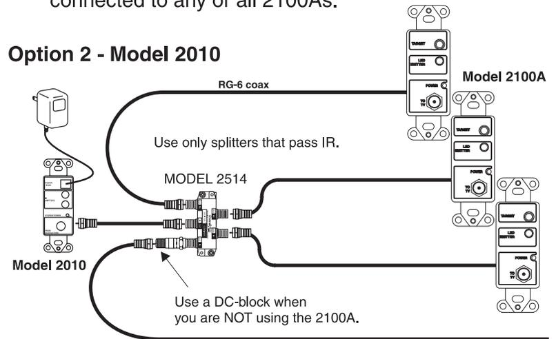
Terminating unused outputs is optional. If you choose to terminate, use only F terminators with a DC block. Otherwise, you will short out the IR engine and trip the internal circuit breaker. (Remove power to reset circuit breaker.)
