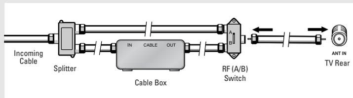
After you've made this connection, set the A/B switch to the "A" position for normal viewing. Set the A/B switch to the "B" position to view scrambled channels. (When you set the A/B switch to "B", you will need to tune your TV to the cable box's output channel, which is usually channel 3 or 4.)
