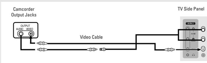
The audio-video cables shown here are usually included with a Camcorder. (If not, check your local electronics store.) If your camcorder is stereo, you need to connect a set of two cables.
