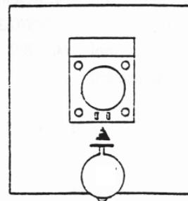
Flap flips up to cover hole when unit is not in use.
