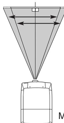
Use LENS SHIFT button and POINT LEFT/RIGHT button to move image left or right. (Refer to page 23.)
