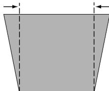
Reduce lower width with KEY STONE ▼ button or POINT DOWN button.
