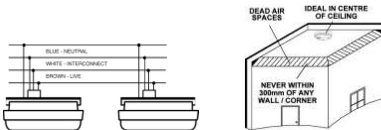
Be very careful about correctly wiring the alarms as mixing Live and Neutral will blow/damage interconnected alarms.
