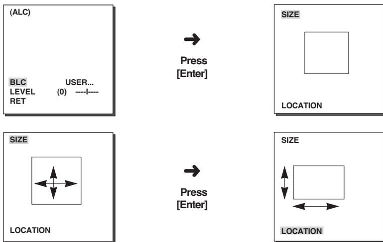
Use [Left, Right] key in the LEVEL menu to control the video output level(brightness).
