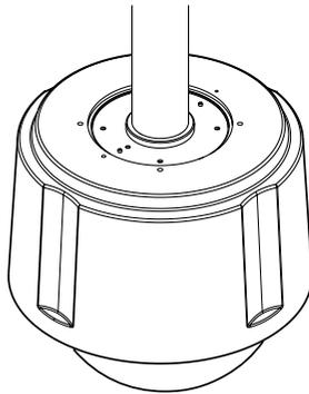
**\* To install and use OUTDOOR HOUSING, remove the Clear Case from the Camera body before installation.**
