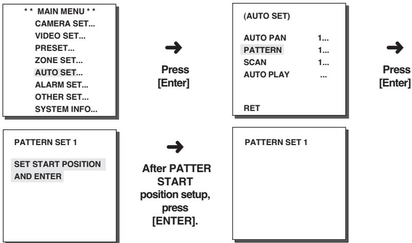
PATTERN can be set upto 3. Choose 1, 2, or 3 with the left or right key in the "PATTERN SET" and press [ENTER] to get into the PATTERN set up screen. From the moment "PATTERN 1 SET" is gone for 2 minutes, it memorizes the MANUAL movements and after 2 minutes it will return to a higher menu. If you want to finish set up before the 2-minutes ends, press [ENTER].
