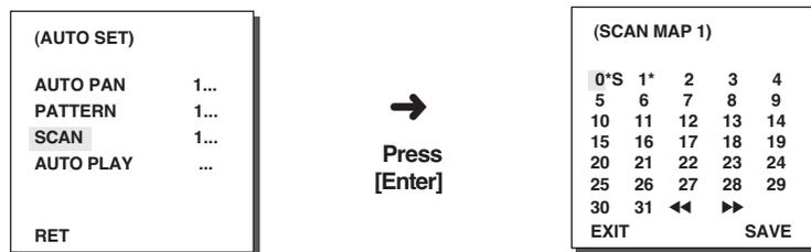
If you enter the SCAN SET screen, SCAN MAP will be displayed. Move the cursor to the number marked \* where PRESET is saved and press [ENTER] and S will appear and a PRESET will be included in SCAN.
