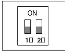
As it is shown in the structure map, when Controller and RS-422A/RS-485 is connected it should be terminated according to the Cable feature of impedance on the each end of the transmitting line to transfer the signals in long distance by controlling the reflection of the signals to the lowest.
