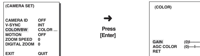
**BW** : The IR Filter is OFF and the screen is black and white. (Sensitivity to low light is increased to a level comparable to a black and white camera.)
