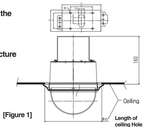
2. Make a hole in the ceiling where the camera will be installed.
