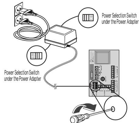
4. **Adjust the switch below the Power Adapter to the proper voltage.** Then, connect the Power Adapter's plug to the Power Connector.
