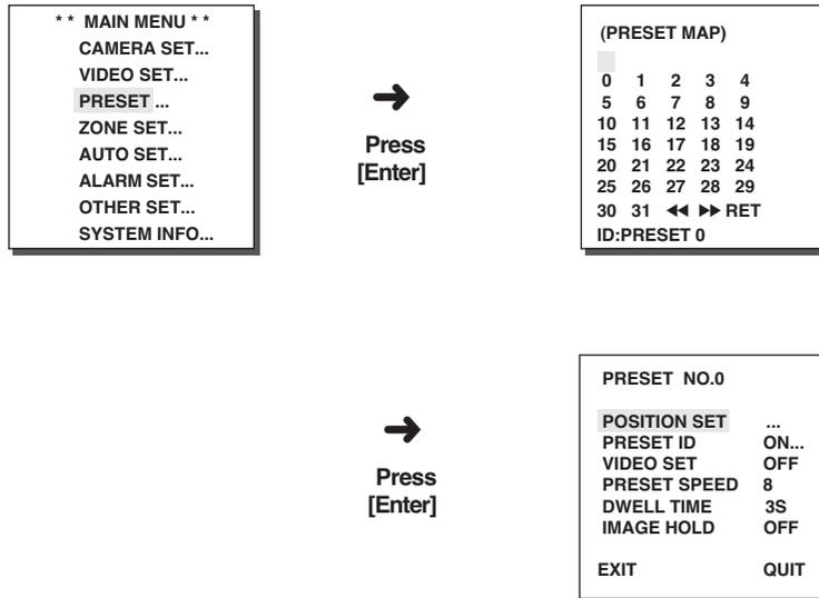
※ Set the PRESET position at the TILT which ranges from 0° to 90°. Beyond this range, PRESET setup is not available.
