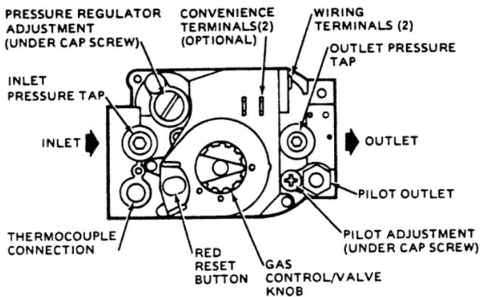
Figure 17 - VR204A /VR8304A Automatic Gas Valve
