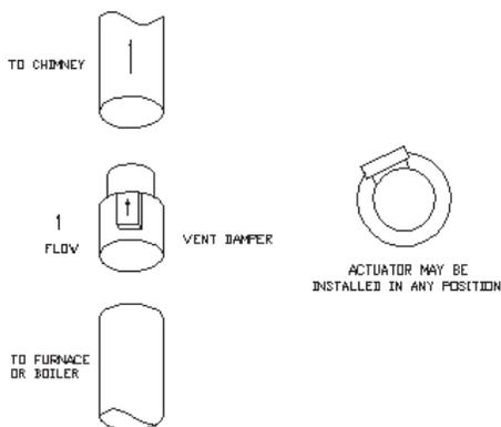
**Figure 7 - Alternate Vent Damper Installation**
