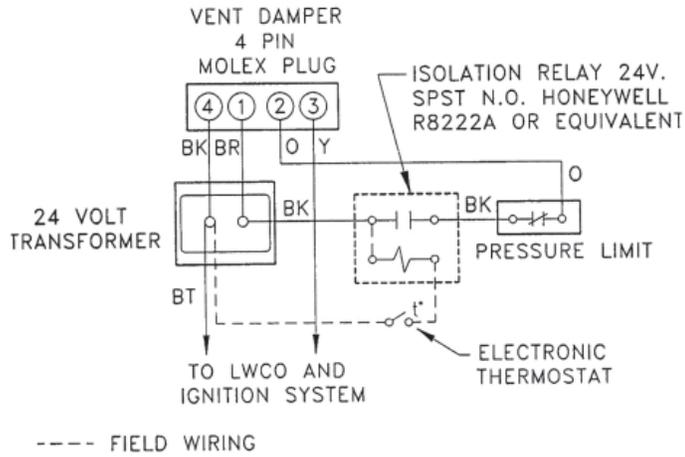
**Figure 10B - Isolation Relay Wiring For Steam Boilers With Probe Type Low Water Cut Off And Using An Electronic Thermostat**
