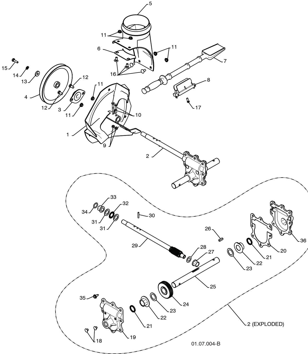
**REPAIR PARTS****AUGER HOUSING / IMPELLER ASSEMBLY****SNOW THROWER - MODEL NO. 1130SB (96193004300), PRODUCT NO. 961 93 00-43**
