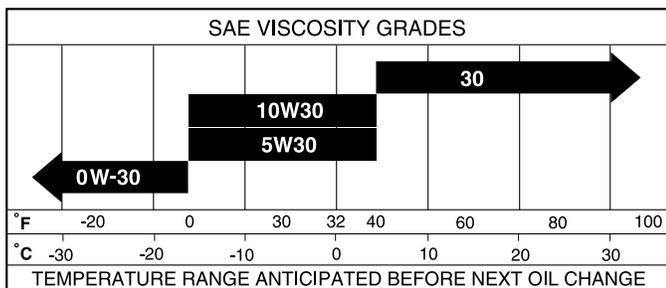
**NOTE:** Although multi-viscosity oils (5W30, 10W30 etc.) improve starting in cold weather, these multi-viscosity oils will result in increased oil consumption when used above 32°F. Check your engine oil level more frequently to avoid possible engine damage from running low on oil.
