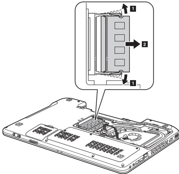
**Note:** If only one DIMM is used on the computer you are servicing, the card must be installed in SLOT-0 ( **a** : lower slot), but not in SLOT-1 ( **b** : upper slot).
