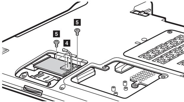
In step **4**, unplug the jack by using the removal tool antenna RF connector (P/N: 08K7159), or pick up the connector with your fingers and gently unplug it in the direction shown by the arrow.
