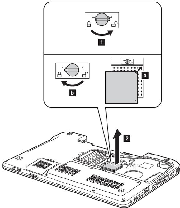
**When installing:** Place the CPU on the CPU socket in the direction shown by arrow **a**, and then rotate the head of the screw in the direction shown by arrow **b** to secure the CPU.
