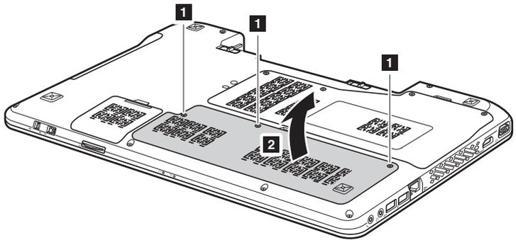
Figure 3. Removal steps of HDD slot cover and HDD (continued)
