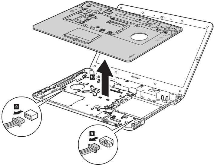
**When installing:** Make sure that the two connectors are attached firmly.
