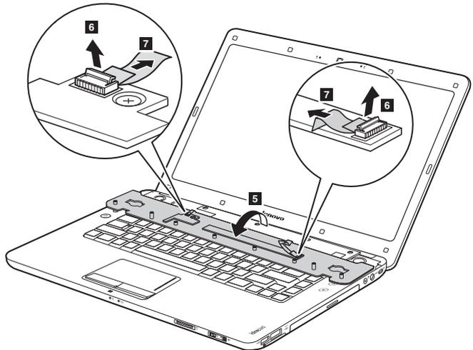
**When installing:** Make sure that the FPC connectors are attached firmly.
