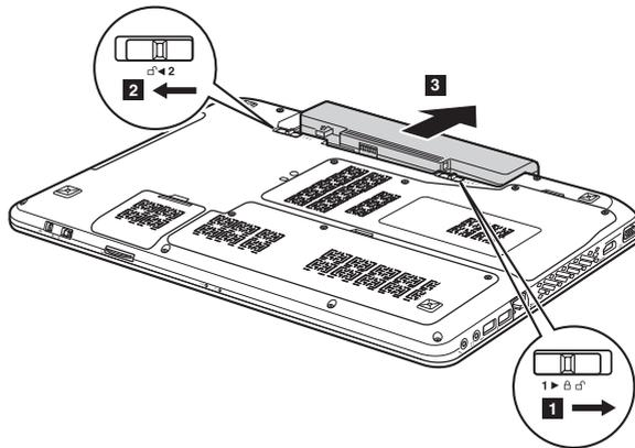
**When installing:** Install the battery pack along the slide rails of the slot. Then make sure that the battery release lever is in the locked position.
