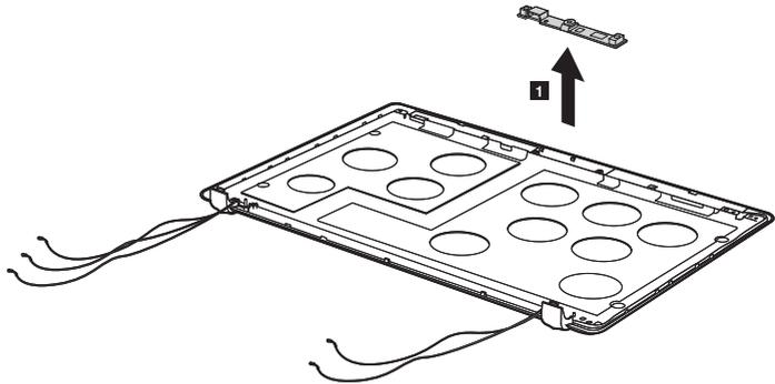
**When installing:** Stick the integrated camera to the top center of the LCD cover and adjust the placement of it to make sure the connector is attached firmly.
