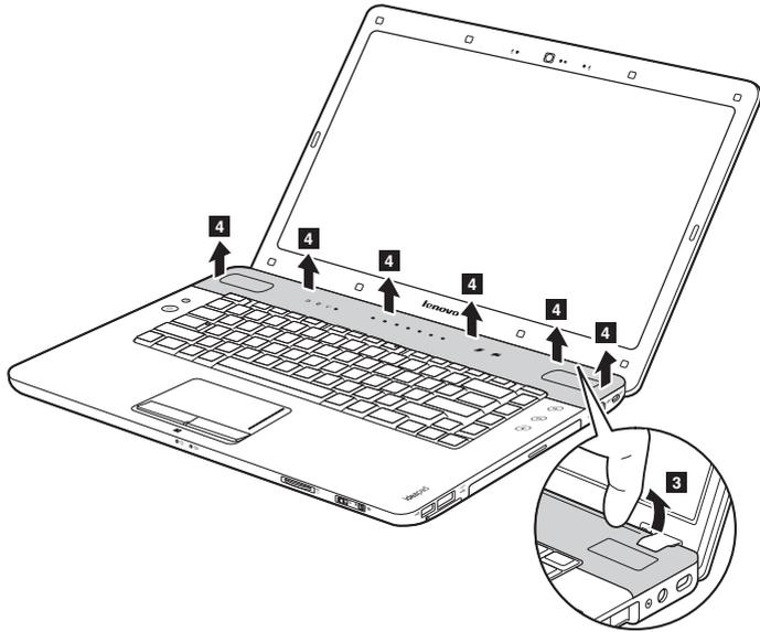
Figure 12. Removal steps of keyboard cover, system status indicator board and touch inductive panel (continued)
