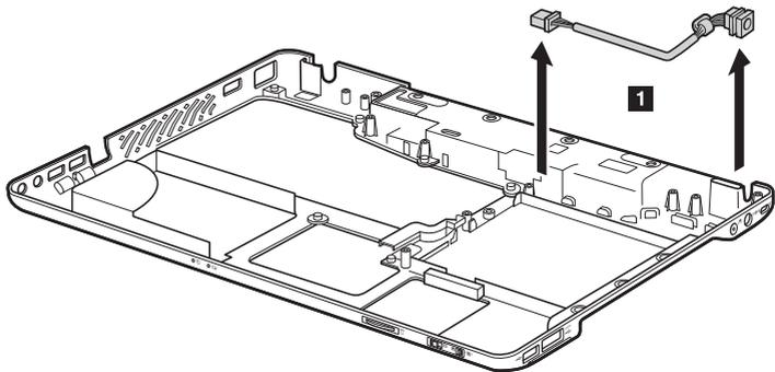
**When installing:** Make sure that the power connector is attached firmly.
