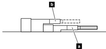
**When installing:** Insert the notched end of the DIMM into the socket. Push the DIMM firmly, and pivot it until it snaps into the place. Make sure that it is firmly fixed in the slot and difficult to be moved.
