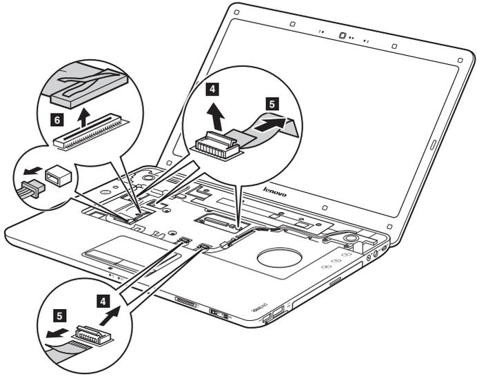
**When installing:** Make sure that all the FPC connectors and the LCD connector are attached firmly.
