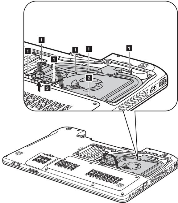
**When installing:** Make sure that the fan connector is attached firmly to the system board.
