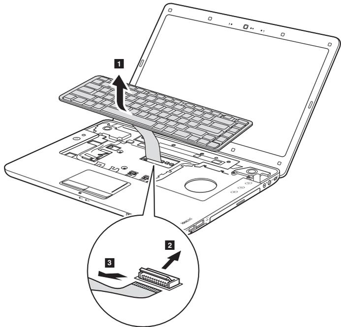
**When installing:** Make sure that the FPC connector is attached firmly.
