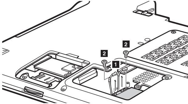
Disconnect the two wireless LAN cables (black, white) ■, and then remove the screws ■.
