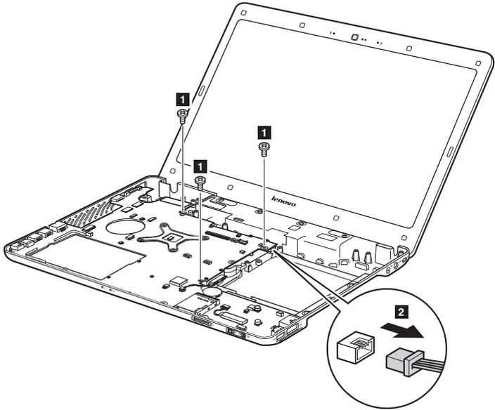
**When installing:** Make sure that the power assembly connector is attached firmly.
