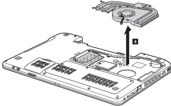
**Attention:** Do not handle the heat sink assembly roughly. Improper handling can cause distortion or deformation and imperfect contact with components.
