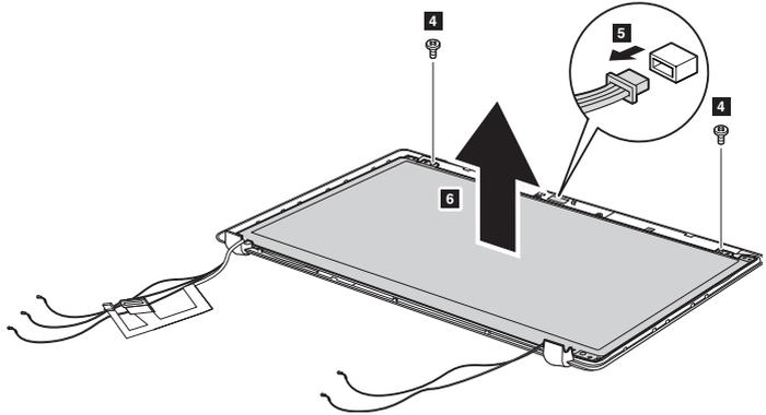
**When installing:** Make sure that the connector is attached firmly.
