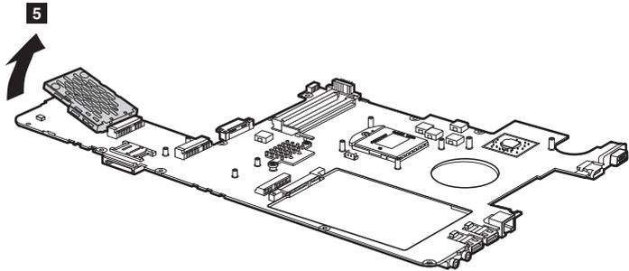
Figure 15. Removal steps of system board, ExpressCard slot assembly and bluetooth daughter card (continued)
