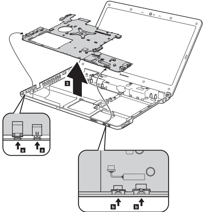
**When installing:** When attaching the system board to the base cover, adjust the placement of the wireless radio switch and the graphics switch as shown in **b**, and make sure that both of the audio jack and the microphone jack are attached to the holes on the base cover as shown in **a**. Improper placement of the switch or those jacks might cause a damage.
