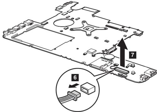
**When installing:** Make sure that the connector is attached firmly.
