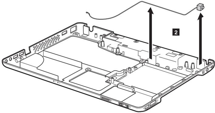
**When installing:** Make sure that the TV-in connector is attached firmly.
