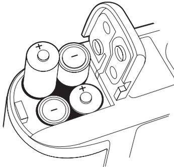
Make sure the + and – terminals are oriented correctly as shown inside the battery compartment. Do not mix old and new batteries, or batteries of different types.
