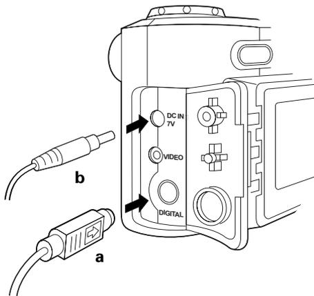
**Note:** Insert the connector straight into the digital port without twisting, so that the flat side of the connector (the side with the arrow on it) faces toward the back of the camera. If you encounter resistance, do not force the connector, but reposition it and try again.
