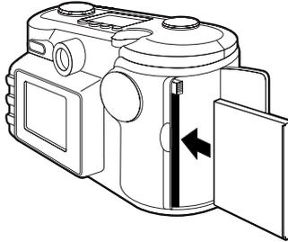
Push the card carefully, but firmly, into the slot. The card fits completely into the slot in only one way. When it is inserted correctly, the eject button above the card pops out.
