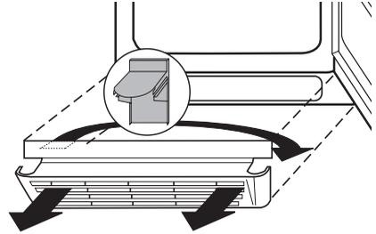
2. With the door closed, remove the cross-head screws from the lower door bearing and remove the door bearing downwards.
