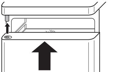
7. Place the lower door bearing with the bearing pivot in the lower left of the door and fasten.
