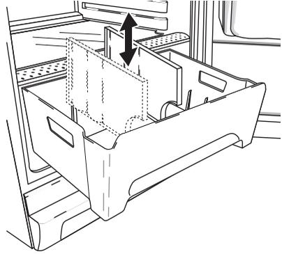
2. If the large divider is inserted in the middle of the bin the right hand side can be further divided by inserting the small divider in the middle or rear position.
