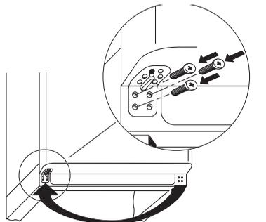
8. Move the door handle from the left to the right and cover the remaining holes with the blanking plugs attached.
