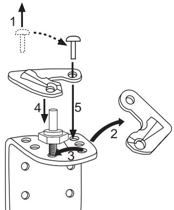
4. Remove the door fitting on the lower right (1) and reposition the door bearing cover from the lower left to the right of the door (2), place the door fitting supplied in the lower left of the door (3). Carefully remove the door to the front and place on one side.
