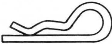
the smallest of three Retainer Springs found in bag of parts. Install Belt Tightener Link through opening in Idler Shaft Assembly. Attach bent end of Link to rear end of Belt Tightener Lever Arm. Secure Retainer Spring (Fig. 4 - left hand inset).
