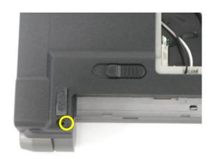
5. Remove 2 screws(M2\*8L(K)) on both ends
