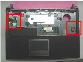
2. Remove 8 screws (M2\*4L(K)) on the top case and 8 screws (M2\*4L(K) on the bottom case.
