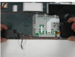
5. Disconnect touch pad FPC cables and remove 5 screws(M2\*3L(K)) then take touch pad backet off and take touch pad away.
