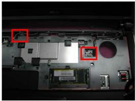
4. Remove 2 screws(M2\*8L(K)) on bottom case
