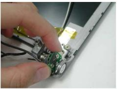
9. Secure 1 screw(M2\*4L(K)) on left and right side hing, then take right and left hinge off.
