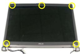
2. Prying the inside edges of the top front bezel, then separate it from LCD back cover and take
