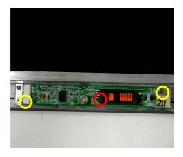
5. Remove 8 screws(M2\*4L(K)) and take the LCD panel off.
