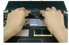
2. Remove Coaxial cable and inverter cable
