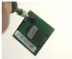
Note: If thermal module has no thermal pad on it, please plus a thermal pad on the CPU die before assembling.
