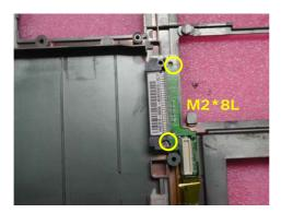
6. Remove the power cable and 1 screw to remove the DC-in jack board.
