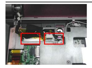
3. Remove Antenna and switch cable.
