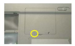
Remove 2 Antenna cables from Wireless LAN Module
