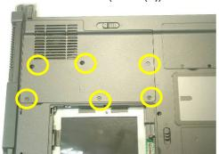
2. Disconnect the FAN connector and remove 2 screws(M2\*4L(K)) then take away the Fan Module.
