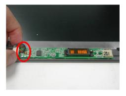
4. Remove 1 screws (M2\*4L(K)) and 2 screws (M2\*3L(K)) take Inverter board off.
