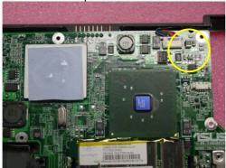
2. Remove 3 screws (M2\*4L(K)) and take away the Motherboard Module from the left side.
