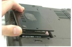
2. Lift the hard disk module and disconnect the FPC then take away the hard disk module.
