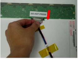
7. Finally, Remove 4 screws(M2\*3L(K)) on the right LCD bracket , and 4 screws on the ilft side to disassemble LCD brackets.
