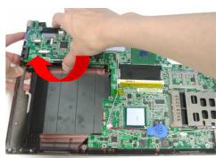
3. Turn the mother board around, remove 2 screws (M2\*4L(K)), disconnect the modem cable.
