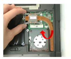
4. Turn the non-removable screw here 180 degrees counter-clockwise to loosen the CPU and take the CPU away
