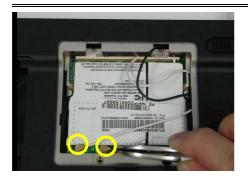
3. Remove the Wireless LAN module by opening the 2 latches aside, which will pop the module up to an angle of 30°, then pull out the module in that angle just like memory module.
