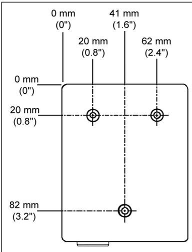
Each IS6520/MS6520 Cubit<sup>®</sup> is equipped with three threaded mounting holes located on the back of the scanner. The following diagram shows the exact location of each mounting hole. The mounting holes are 6 millimeters deep and are threaded for use with 3 millimeter screws.
