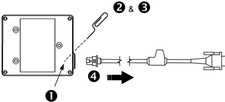
1. Locate the small 'pin-hole' on the back of the scanner.
