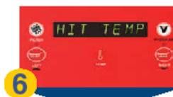
Once the oil level has been checked and verified, press the TEMP button. The burners will automatically turn back on and the fryer will resume heating. **HIT TEMP** displays.
