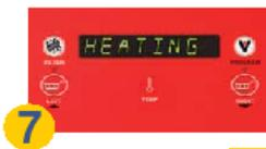
After pressing the TEMP button the fryer resumes heating. **HEATING** displays.
