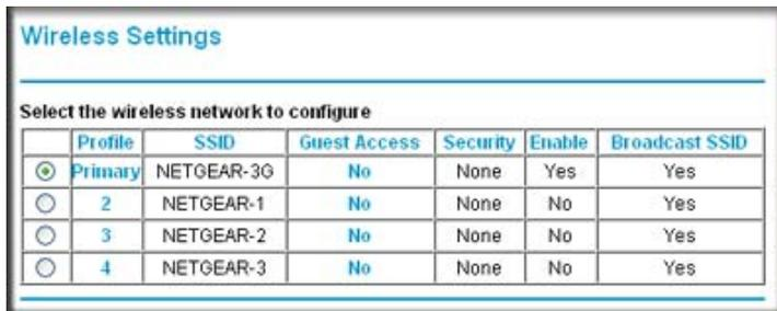
2. Select the radio button for the network profile that you want to set up.
