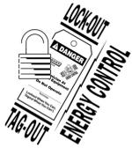
**WARNING** Certain procedures in this section require electrical test or measurements while power is applied to the machine. Exercise extreme caution at all times and follow Arc Flash procedures. If test points are not easily accessible, disconnect power and follow Lockout/Tagout procedures, attach test equipment and reapply power to test.
