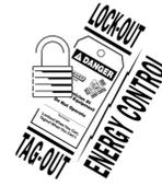
**WARNING** Disconnect the electrical power to the machine and follow lockout / tagout procedures.
