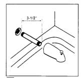
3 After wall is finished, install 1/2" nipple to extend 3-1/2" beyond finished wall. Install spout.
