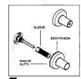
1 Screw plastic sleeve onto threads at base of stem. Place ring of putty underedge of escutcheon. FINGER tighten escutcheon onto sleeve securely against wall.
