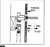
2 Position valve body so distance between center of supply lines and finish surface of wall DOES NOT EXCEED min. or max dimensions.
