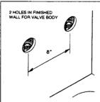
1 Make two 2" diameter holes in wall on 8" centers. Position supply lines at hole
