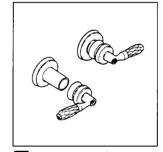
2 Attach both handles with handle screws provided. Snap index button into each handle.
