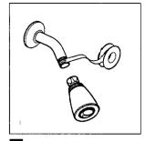
4 Make 7/8" hole for shower arm. Slide flange on to arm and thread arm into I.P. elbow. Slide flange against wall. Attach showerhead to arm with teflon tape. Hand tighten. If wrench is used, protect chrome finish.
