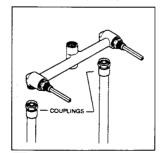
3 Connect couplings to hot and cold supply lines using thread sealant or teflon tape on pipe. Connect valve body to hot and cold supplies using 1/2" couplings.
