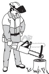
**When the bar hits the stump the brake should be applied.**
