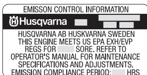
The Emissions Compliance Period referred to on the Emission Compliance label indicates the number of operating hours for which the engine has been shown to meet Federal emissions requirements.
