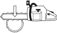
Finish by cutting from below so that the two cuts meet.
