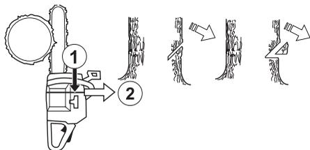
The directional cuts should run 1/4 of the diameter through the trunk and the angle between the top cut and bottom cut should be 45°.
