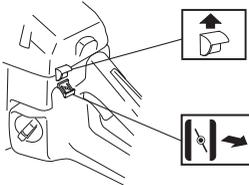
**Primer bulb:** If the machine is fitted with an air purge (A): Press the air purge repeatedly until fuel begins to fill the bulb. The bulb need not be completely filled.
