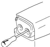
Some mufflers are equipped with a special spark arrestor screen. If your machine has this type of muffler, you should clean the screen at least once a week. This is best done with a wire brush. A blocked screen will cause the engine to overheat and may lead to serious damage.
