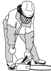
Push in the choke control as soon as the engine fires and make repeated starting attempts. Immediately press and release the throttle when the engine starts. That will disengage the throttle latch.
