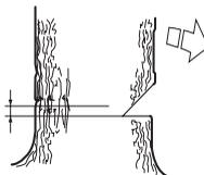
Finish the felling cut parallel with the directional cut line so that the distance between them is at least 1/10 of the trunk diameter. The uncut section of the trunk is called the felling hinge.
