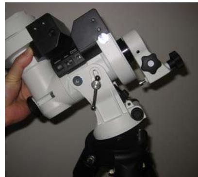
4. **Adjust Latitude:** Slightly loosen the Latitude Locking T-bolts. Turn Latitude Adjust Knob to adjust the latitude until the arrow points to your current latitude on the Latitude Indicator (see 2<sup>nd</sup> photo in step 1). Relock the Latitude Locking T-bolts.
