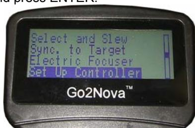
Enter the date and check if it is Daylight Saving Time using arrow keys and number keys. Enter your time zone (add or subtract 60 minutes per time zone) by entering minutes “behind” UT or “ahead” of UT, such as:
