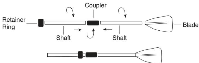
The assembled oar is to be inserted into the oar locks from the outside of the boat. The oar retainer ring is then placed onto the top half of the assembled oar, from the inside of the boat, to prevent the oar from sliding into the water (see below).
