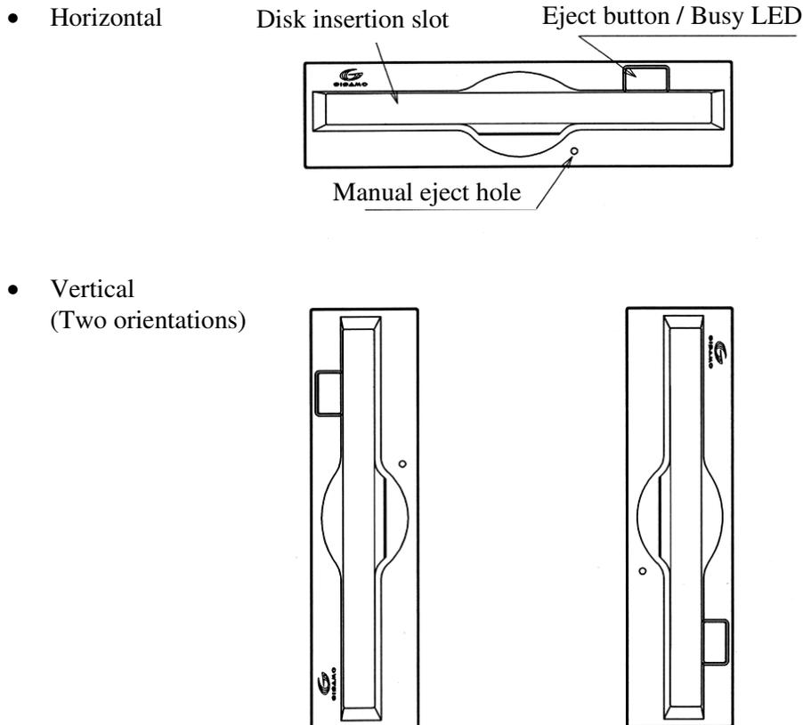
**Figure 5.1 Optical disk drive front view (with panel)**
