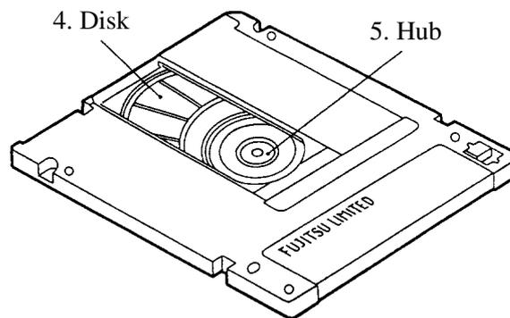
**Figure 5.4** Optial disk cartridge
