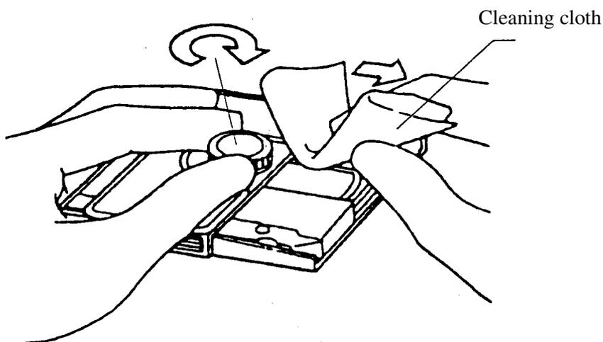
**Figure 5.10 Cleaning procedure (4)**
