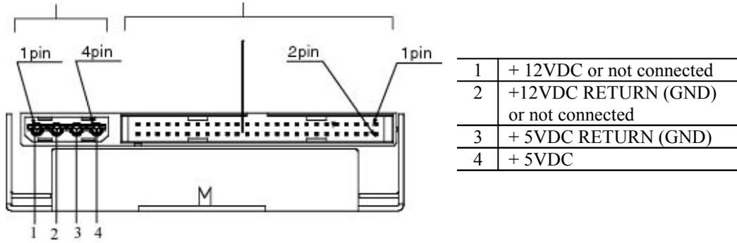
**Figure 3.9 Connector and terminal locations**
