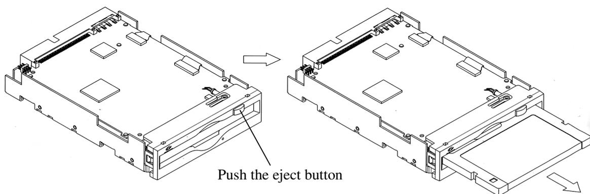
**Figure 5.3 Removing cartridge**
