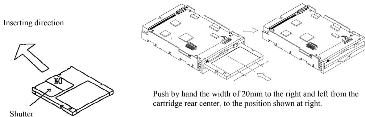
**Figure 5.2 Inserting cartridge**
