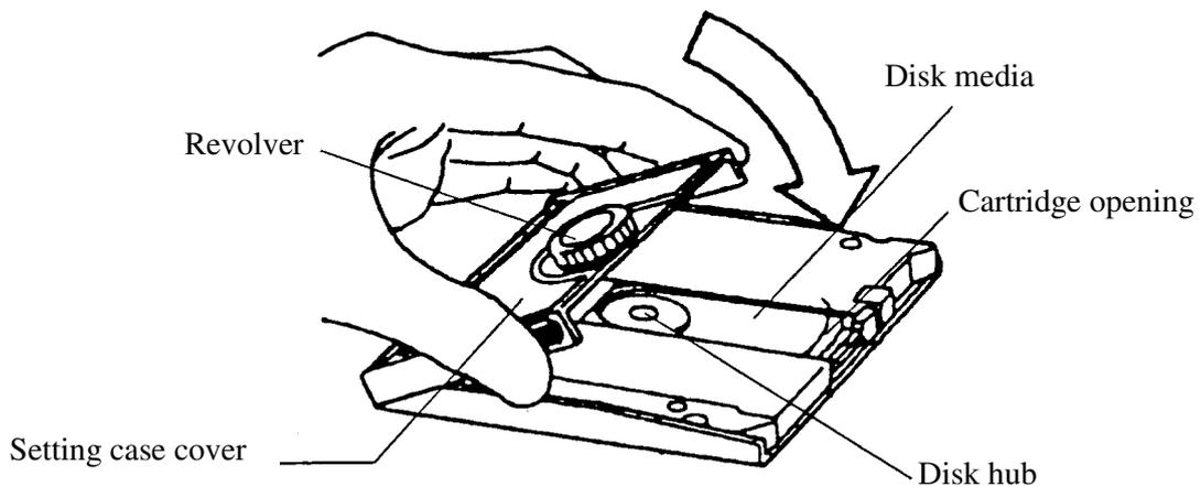
**Figure 5.9 Cleaning procedure (3)**
