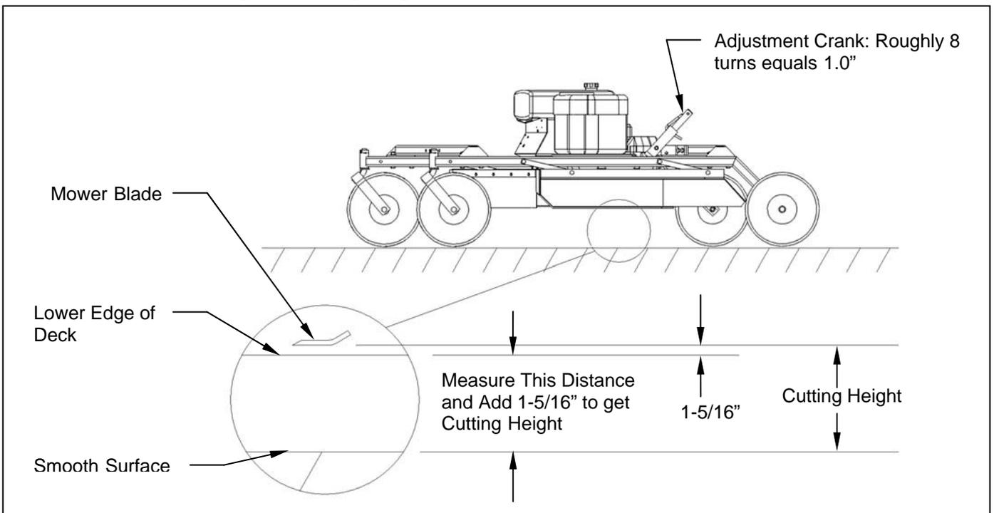
Figure 8: Adjusting Rough Cut Mower Cutting Height
