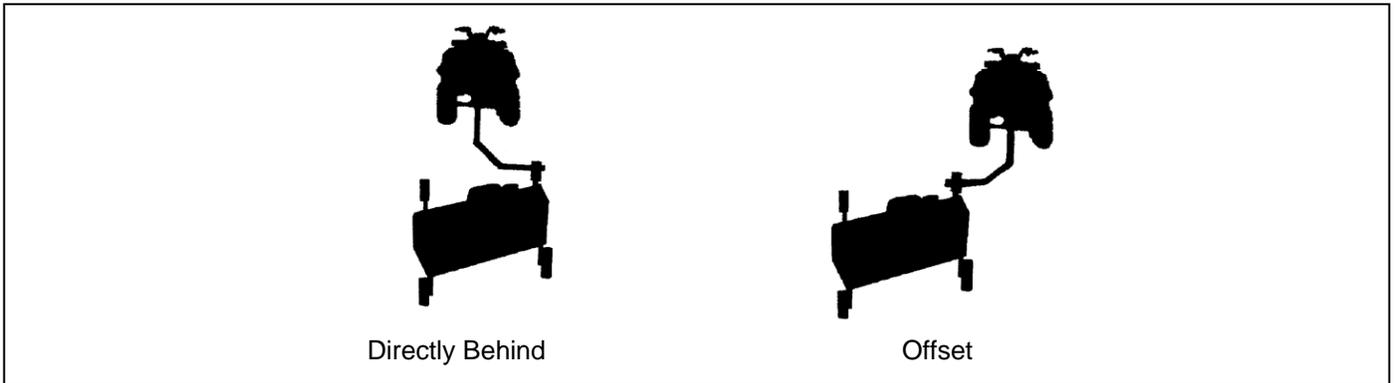
Figure 7: Rough Cut Tow Behind Towing Suggestions
