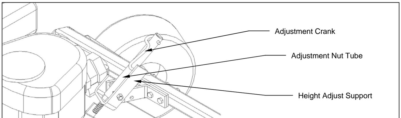
Figure 9: Securing Crank While Not In Use
