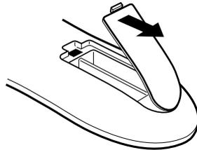
2. Install two "AAA" size batteries. Match the + and - signs on the batteries to the signs on the battery compartment.
