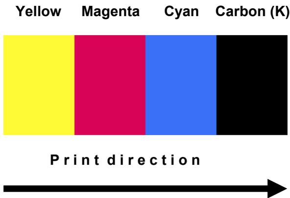
For special needs, we are also offering color ribbons with an additional K field. This is a useful option if e.g. a customer needs to print the front of a card in YMCK while on the back of the card has to be printed only some text information in K. The CMYKK ribbon enables this process without the use of a double patch of YMCK and is very cost saving.
