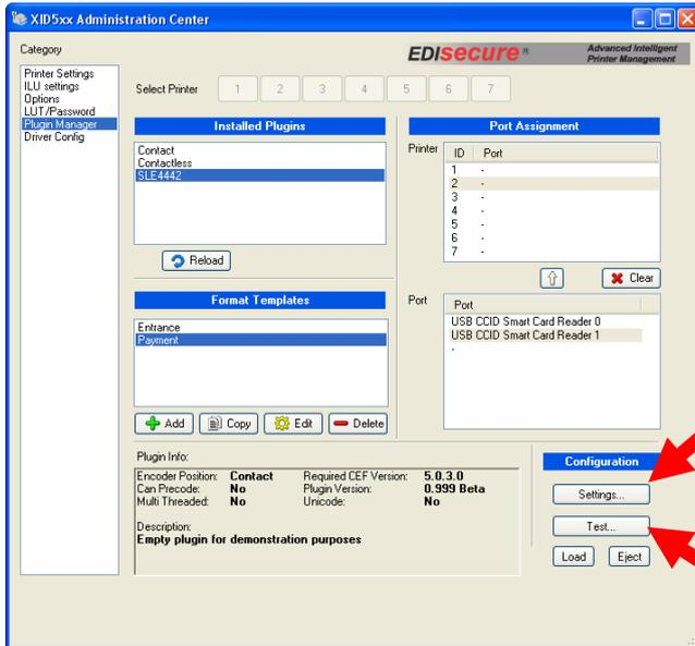
If these options are provided by the plugin, clicking on either button will open a configuration or a test dialog and show the corresponding functions that are necessary to configure the encoder hardware and to test the encoding of the card.
