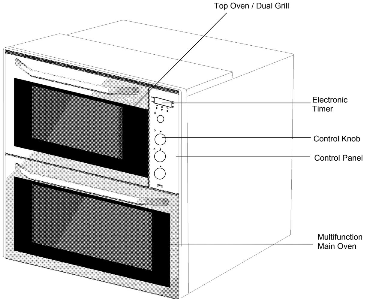
Your built in appliance comprises of a conventional oven and dual grill in the top compartment. The top oven is convenient and economical for mid-week use because of its size.
