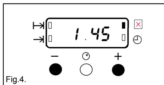
The 'Countdown' will sound intermittently for up to 2 minutes at the end of the timed period. The sound can be stopped by pressing any button.
